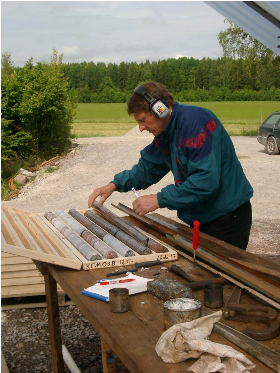
Figure 4-1. Field logging of the drill core is here made on-site by drilling manager Göran Nilsson.
