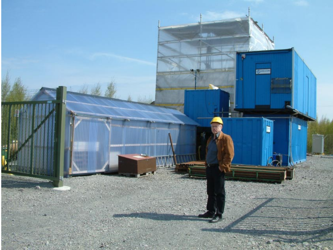
Figure 1-3. Investigation leader Lennart Ekman standing at drilling site DS3 with drill core shelter to the left and a plastic weather protection around the drilling machine.
