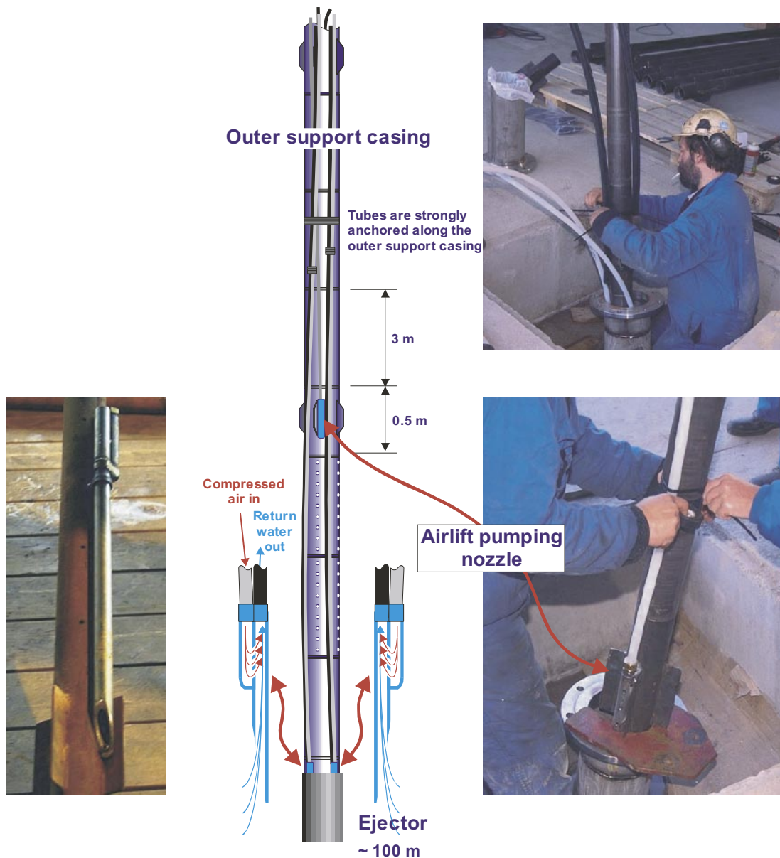
Figure 3-5. Schematic representation of connection and installation of airlift pumping nozzle and ejector on the outer protective casing.
