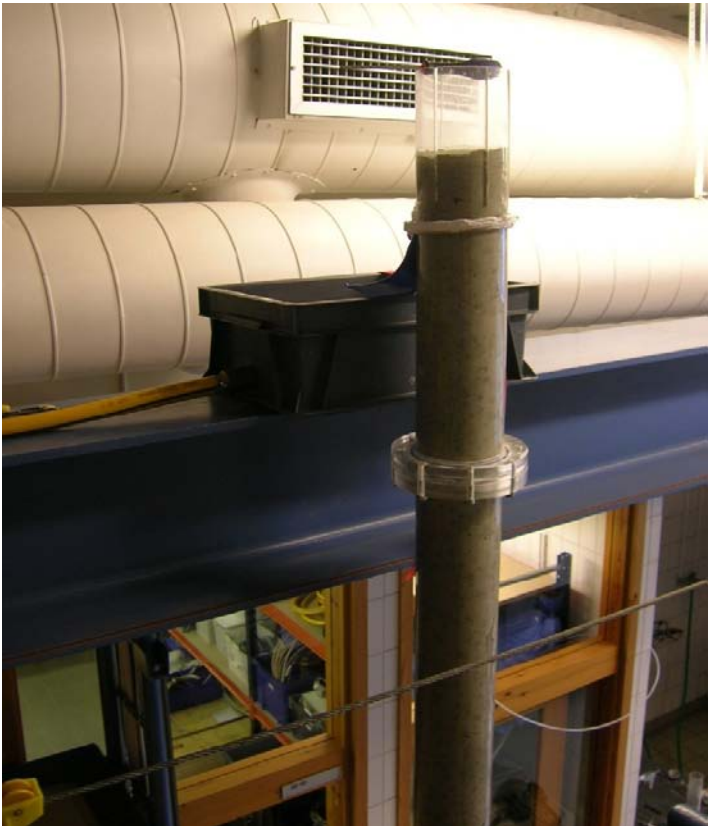
Figure 4-2. Photo showing the upper end of the 4 meter high test equipment where the water was collected.
