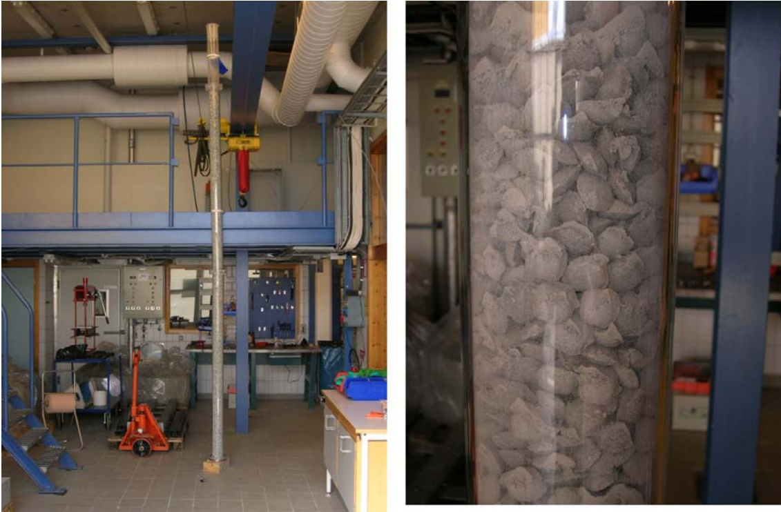
Figure 4-1. Photos showing the test equipment used in the tests. The left photo shows the 4 meter long test equipment. The right photo shows a close up view after filling the tube with pellets.
