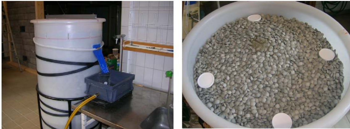
Figure 4-9. Left: Arrangement for collecting water in order to measure the erosion. Right: Pellets surface about 20 hours after test start. Water has entered the surface in the middle. The white plastic lids are placed on the pellets surface measuring movements.
