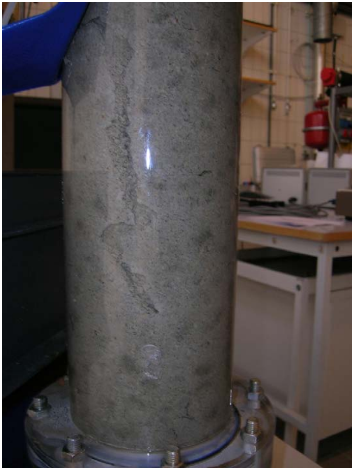
Figure A10-2. The water is flowing in a channel.
