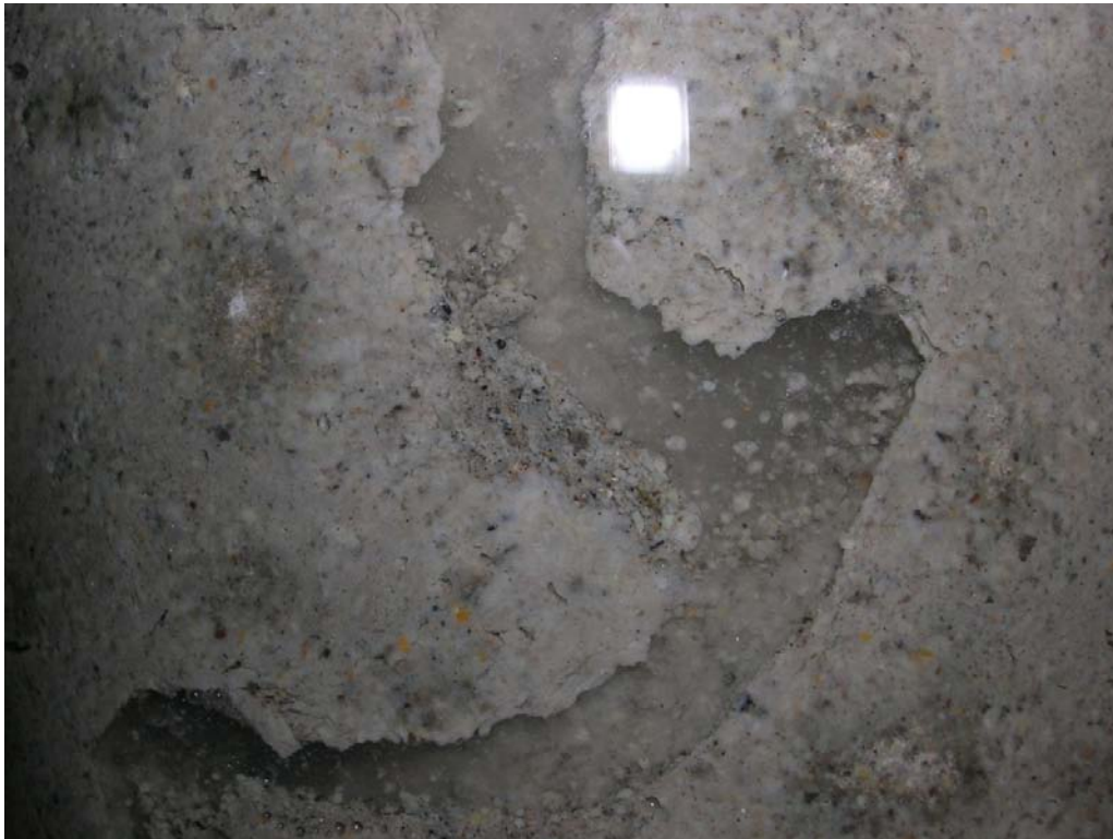
Figure A12-2. In the beginning of the test it is possible to see how material is transported in the channel formed by the flowing water.
