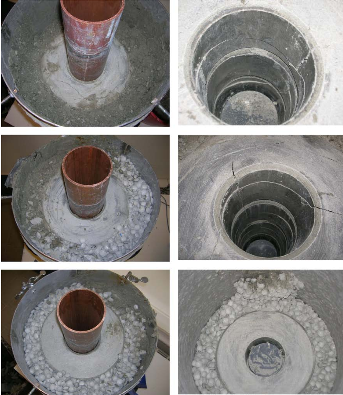
Figure 3-4. Photos taken during dismantling of the tests with different inflow rates. Upper. 0.1 l/min: The whole pellet filling is wetted. There are distinct cracks in the blocks. Middle. 0.01 l/min: Half of the pellet filling is wetted. Also in this test distinct cracks can be seen in the blocks. Lower. 0.001 l/min: Only a small part of the filling is wetted. The water has ascended in a channel along the “rock” wall.
