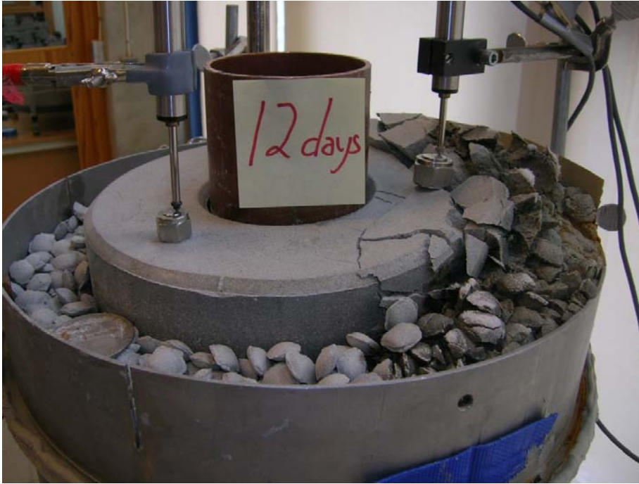
Figure A4-3. Photo taken just before terminating of the test. The upper block and pellets are strongly influenced by the water flow.
