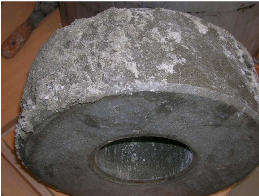
Figure A8-4. Photo taken during excavation. The movements of the blocks have been made by the pellets which have "grabbed" the block surface.
