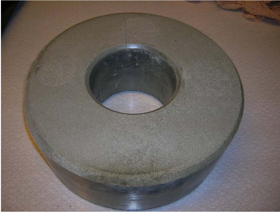
Figure A9-3. The second block from the bottom. One part is affected of water and has swollen 4–5 mm (block thickness). The block has cracked opposite the water inlet.
