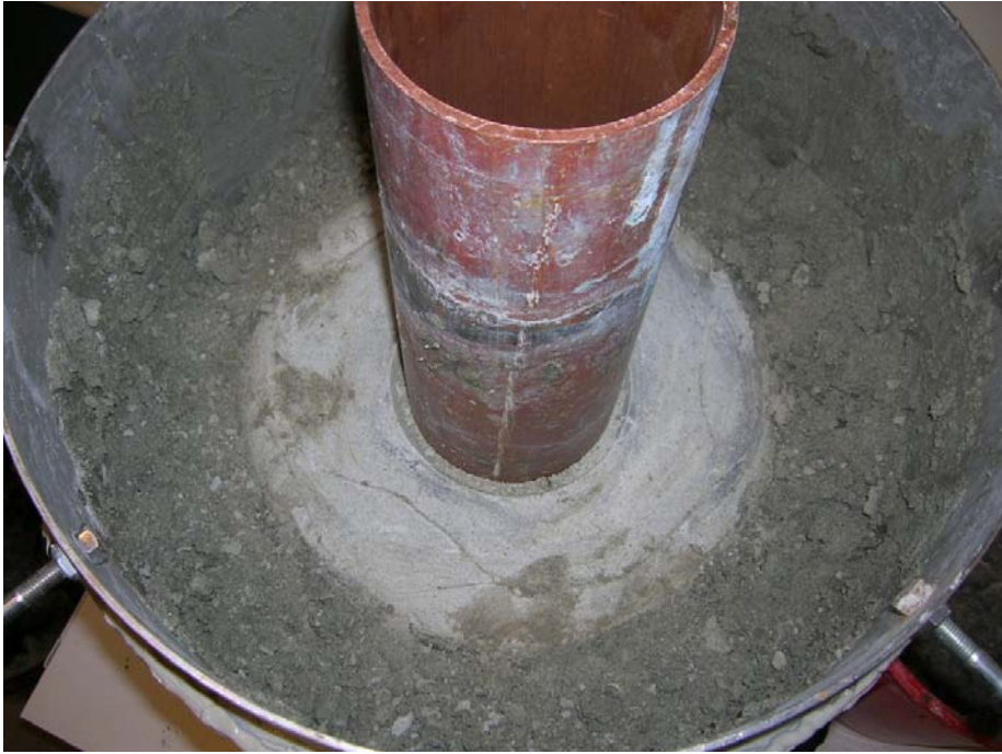
Figure A2-3. Photo taken during excavation. The surface between the blocks is still dry but the pellets are completely wetted.
