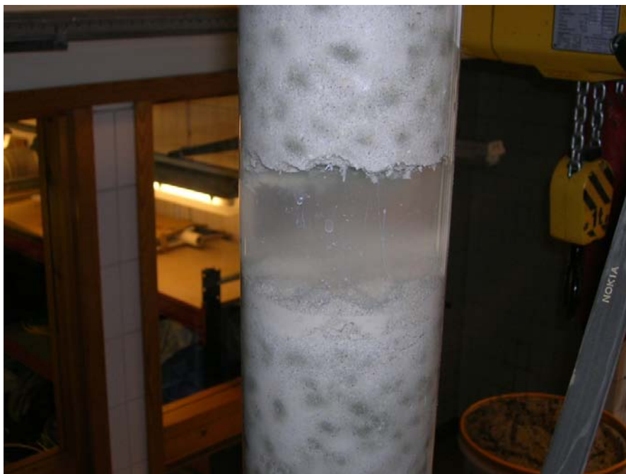
Figure 4-4. When the bentonite had sealed at one level, the water pressure could act on the whole cross section and the pellets column was pushed upwards.
