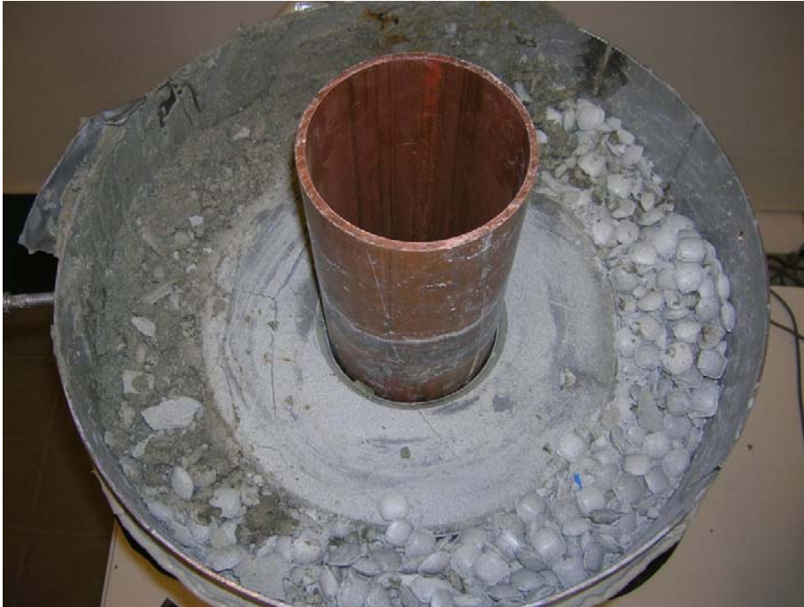
Figure A3-3. Photo taken during excavation. The surface between the blocks is still dry and it is only parts of the pellets filled slot that is wetted.
