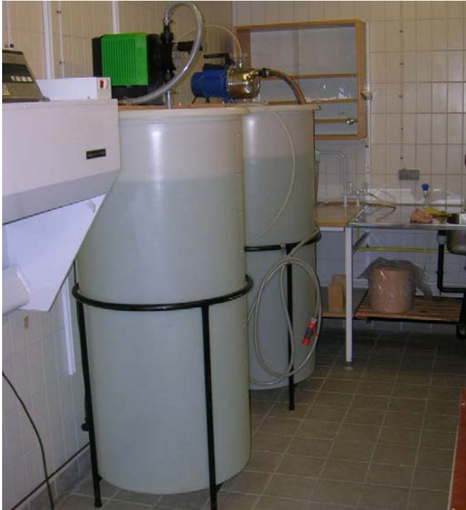
Figure 4-10. Vessels and pumps for mixing and supplying the test device with water.
