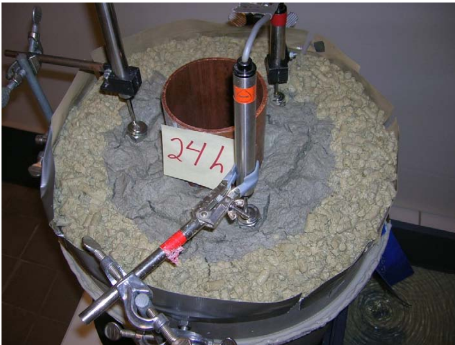
Figure A1-4. Photo showing the upper surface of the test after 24 hours. Water have poured out on the block surface and the bentonite have swollen.
