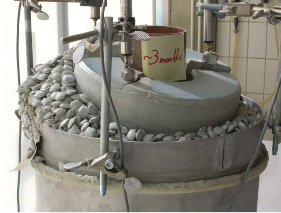
Figure A6-3. After three months test has the uppermost block tilted strongly.
