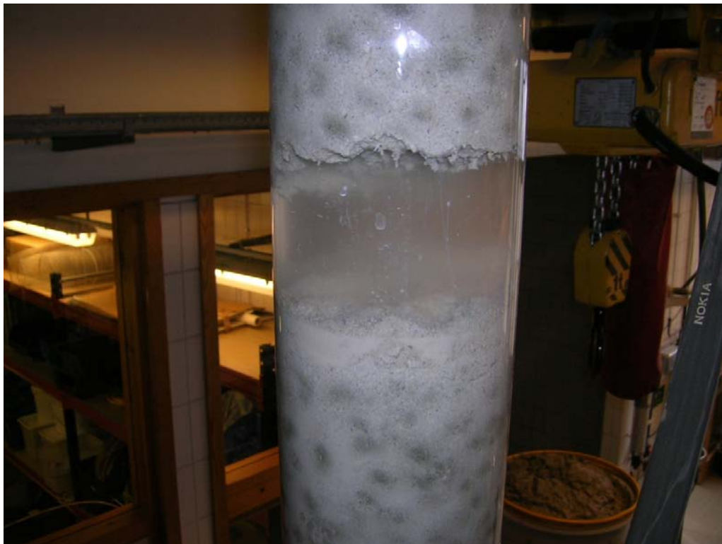
Figure A11-2. The bentonite separates and the water pressure can act on the whole cross section area, pushing the bentonite upwards.
