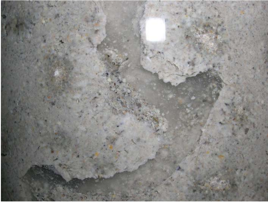
Figure 4-16. In the beginning of a test it is possible to actually see the eroding material. All water seems to flow in one main channel.
