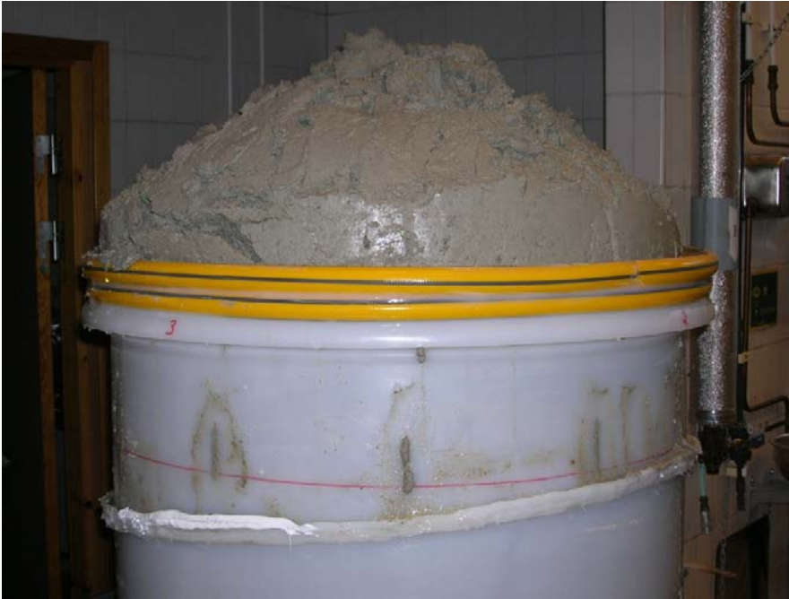
Figure 4-15. After 4 months test duration and measurement of erosion the pellets column rose about 100 mm during a weekend.
