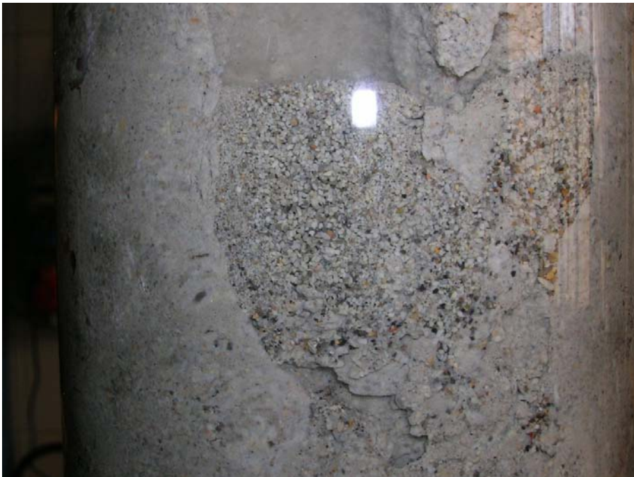
Figure 4-17. Typical whirls with coarse particles that are not transported away with the flowing water.
