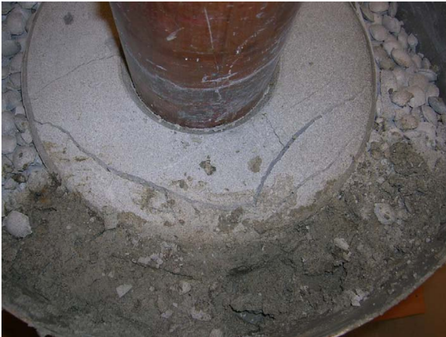
Figure A5-4. Photo taken during excavation. The pellet filling is only partly wetted. There are large cracks in the blocks, mainly on the half closest to the wetted pellets.
