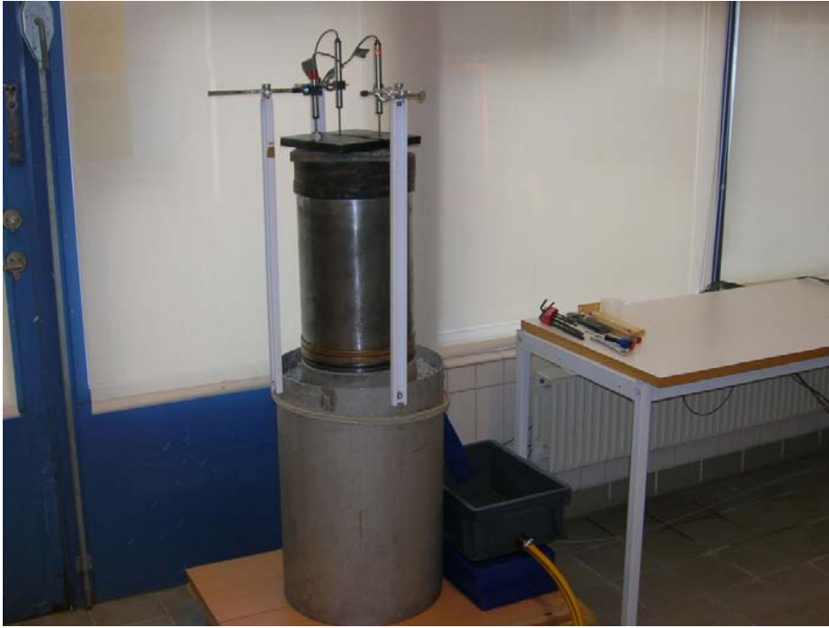
Figure A5-3. Overview of the test layout. Weights are placed on yhe top of the bentonite blocks simulating an overload of 40 kPa.
