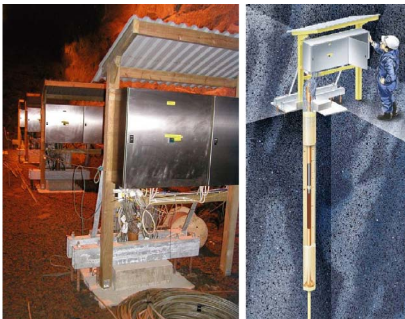
Figure 4-2. Left: Picture of the test site including 4 test parcels and local data collecting device. The data collecting computers were placed in a hut behind the photographer. Right: Schematic drawing of the final appearance of a test parcel after installation.
