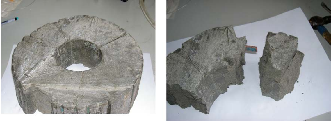
Figure B-2. The received bentonite block A030 to the left and copper coupon A030C visible after breaking apart the bentonite block to the right (item 2).
