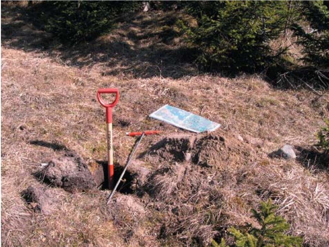
Figure 4-4. Within the areal mapping of Quaternary deposits, pits were dug and surface samples collected for textural and chemical analyses.
