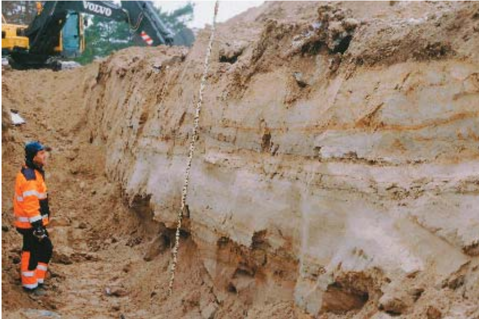
Figure 4-6. One example of a machine-cut trench, studied for seismically induced liquefaction. The trench is c 80 m long, located on the eastern flank of the Börstilåsen Esker. No distinct indications of late or postglacial faulting have appeared so far. The investigations are planned to continue throughout 2004.
