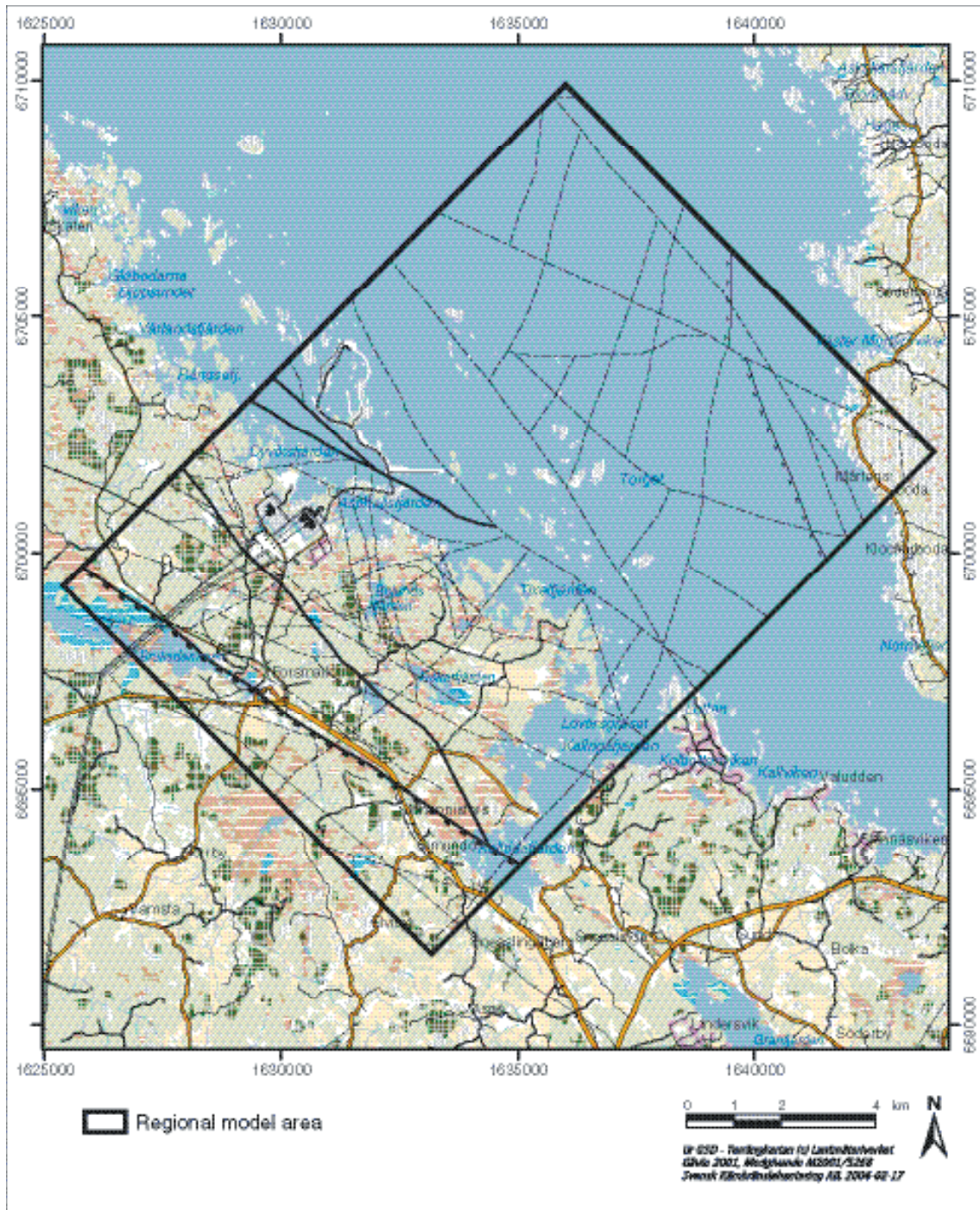
Figure 2-3. Regional model area in version 1.1 (same as in version 0). The depth of the volume is set to 2.2 km. The figure also shows the lineaments (dashed lines) and fracture zones (solid lines) identified in version 0. The selected regional model area captures relevant portions of the regional deformation zones.
