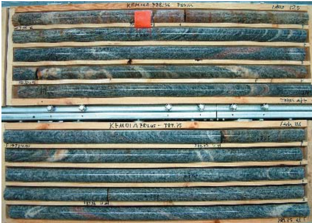
Figure 5-42. Bore core from KFM01A, 778.36–789.75 m. The figure illustrates the geological structures in the rock, such as foliation.
