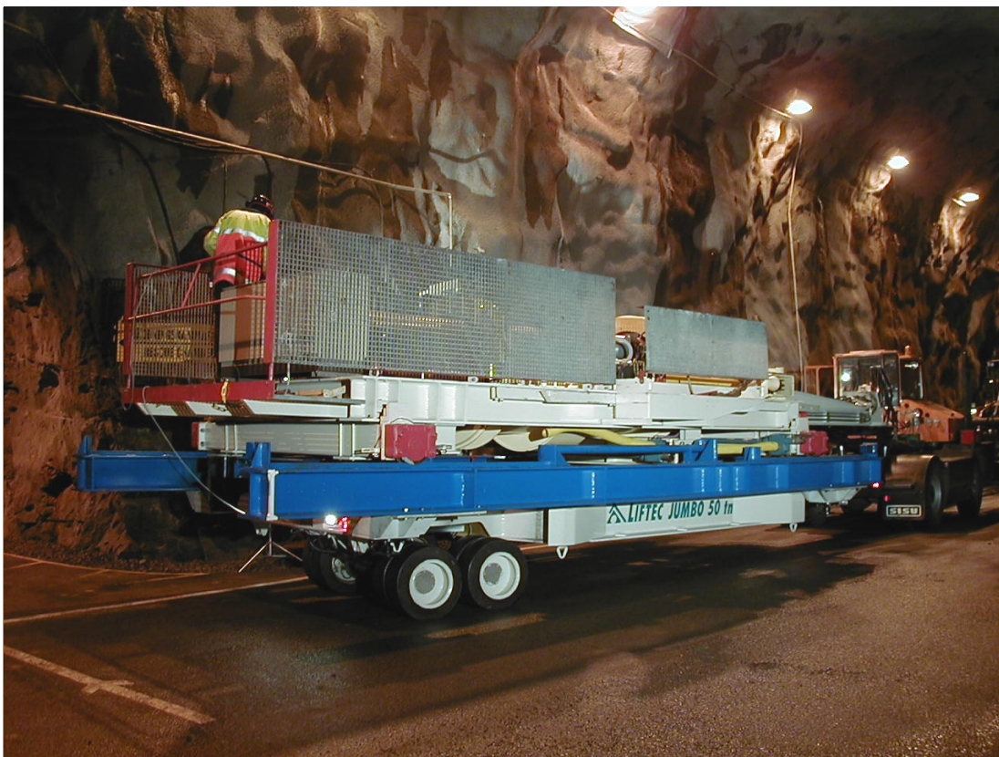
Figure 4-5. The canister and deposition-machine placed on a trailer.
