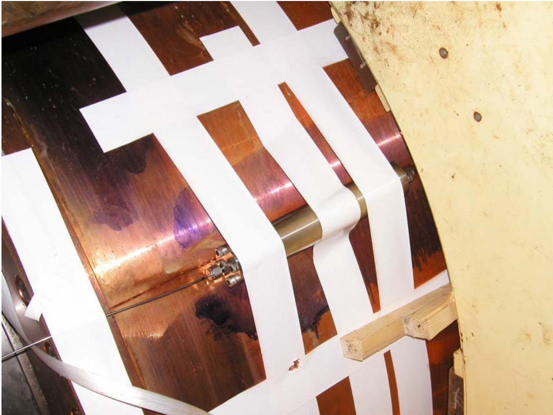
Figure 4-4. The tube with the fixed optical cable placed on the surface of the canister with tape. The tape was removed before the deposition of the canister.
