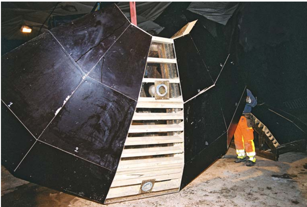
Figure 6-5. The framework of plywood and plexiglass.
