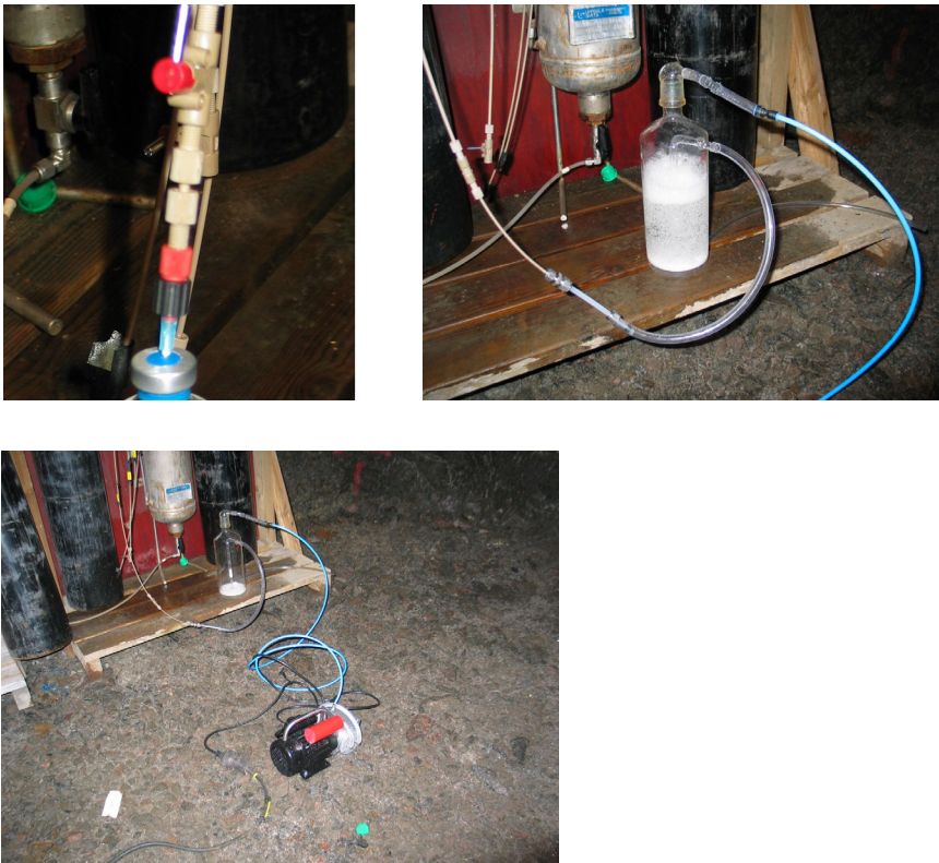
Figure 2-1. The sampling equipment. From left to right: junctions and valve with stopcock, glass flask, vacuum pump.
