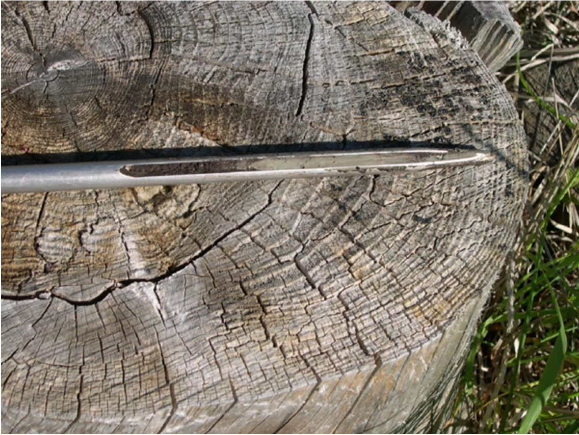
Figure 3-1 b. Sample taken with the hand driven probe.
