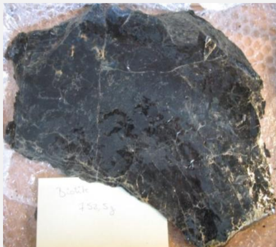
A (25x15 x1 cm) chunk of the biotite sample used in the experiments.
