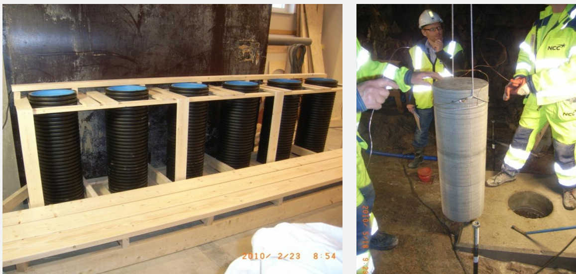
Cylinders used for the experiments (left) and installation of cylinder in a selected hole (right).
