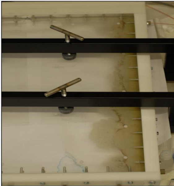
The expansion of bentonite into an artificial fracture.
