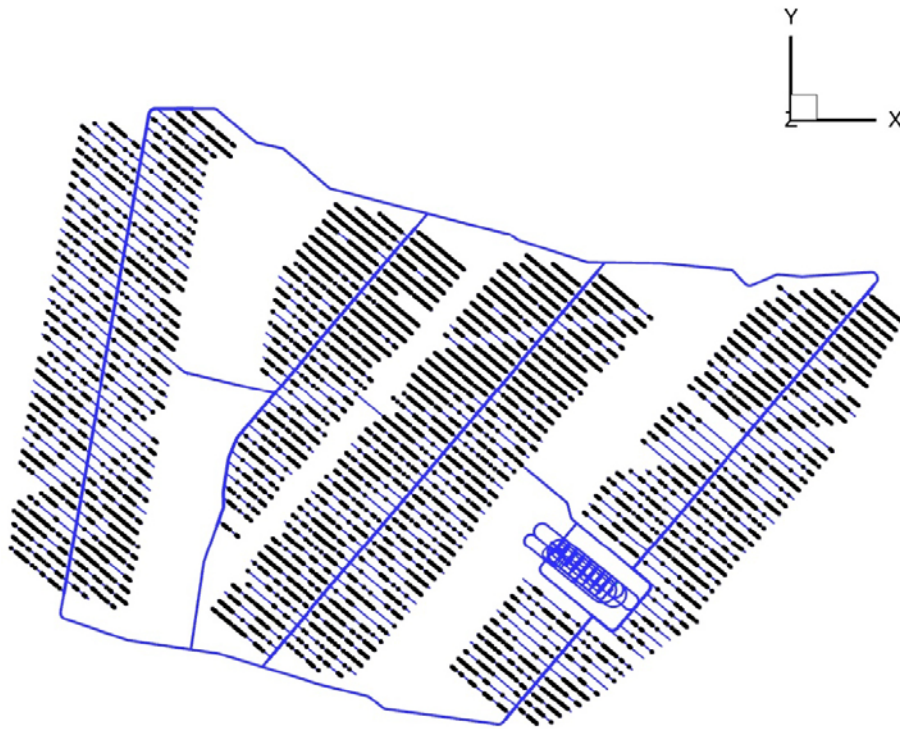
Figure 5-22. Positions of the 5,183 deposition holes that did not pass the \{Q1 \cup Q2\} criterion (Variant III).
