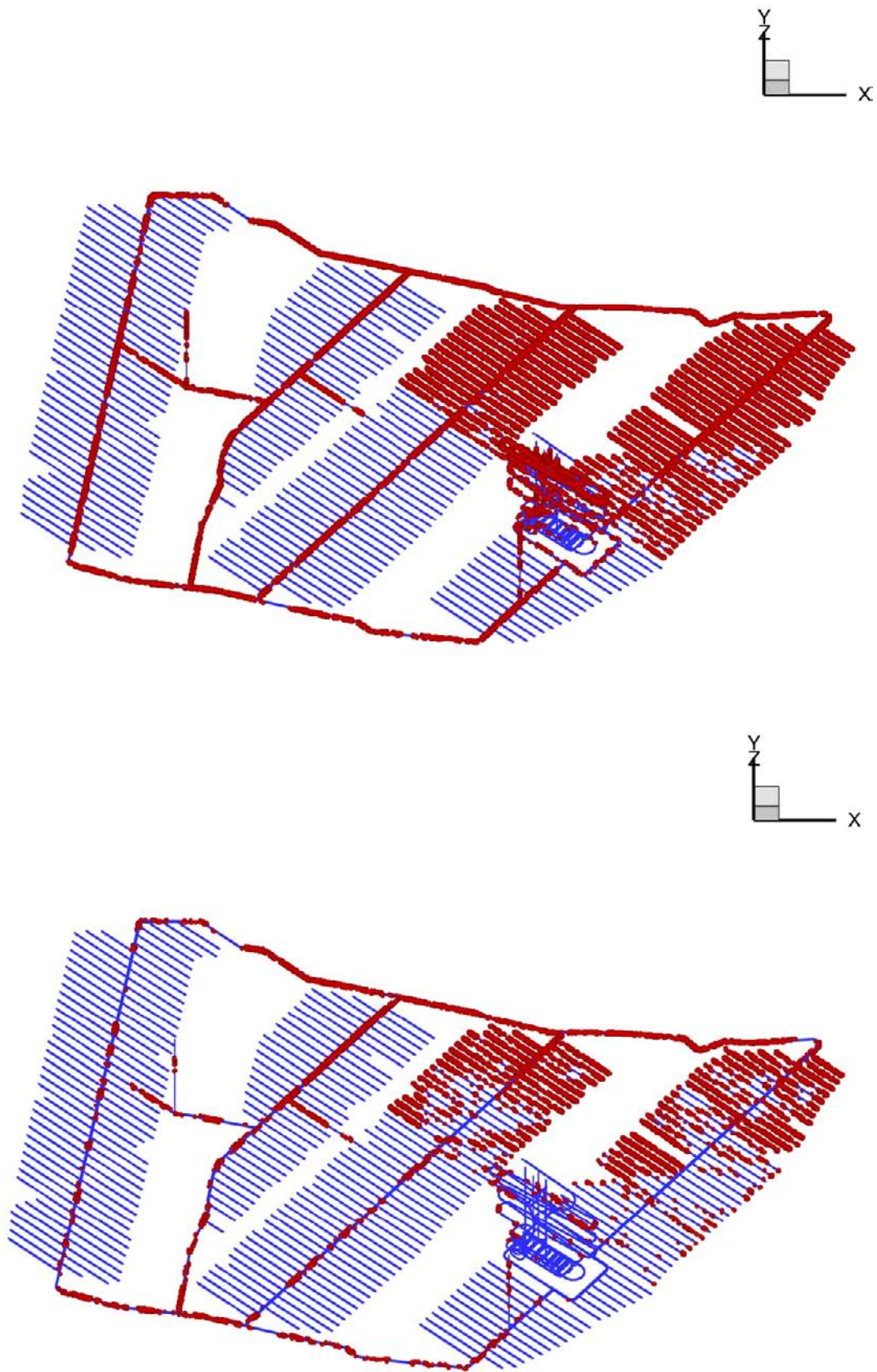
Figure 5-7. Cells with an inflow rate greater than 0.1 L/min (top) and 0.5 L/min (bottom) are marked up by spheres. Operation stage E and grouting level II.
