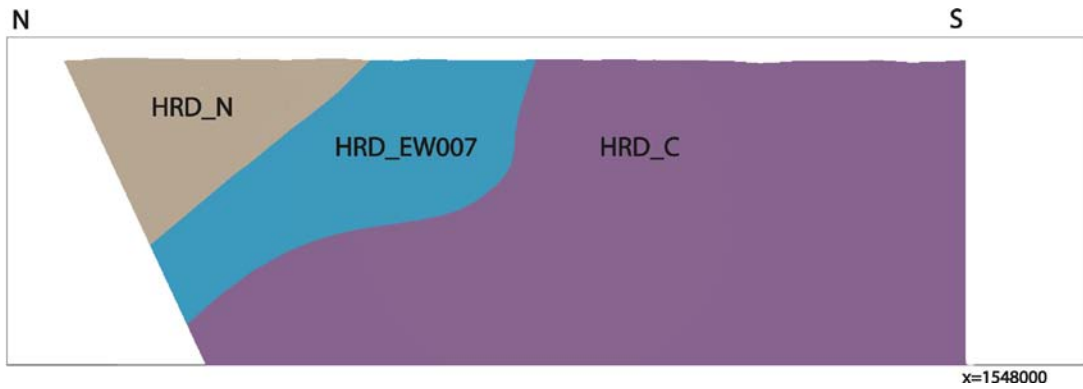
Figure 2-9. Illustration of the SDM-Site Laxemar Hydraulic Rock Mass Domain Model. Vertical section from north (left) to south-at Easting's X = 154,800 m, /Rhén and Hartley 2009/.
