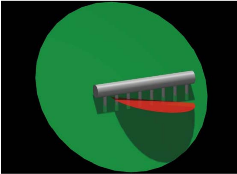
Figure 4-9. Definition of EFPC (Expanded Full Perimeter Criterion). A potentially discriminating fracture can remain undetected despite the use of the FPC in the deposition tunnel. (Figure 5-2 in /Munier 2006/.)
