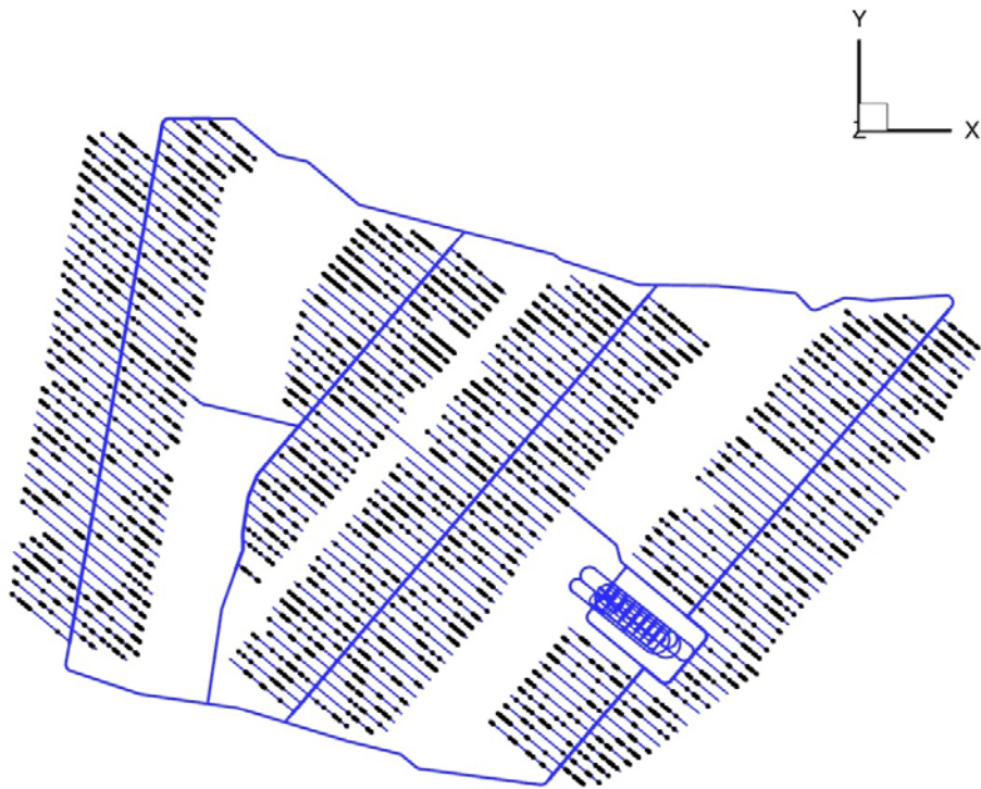
Figure 5-21. Positions of the 2,758 deposition holes that did not pass the \{Q2\} criterion (Variant II).
