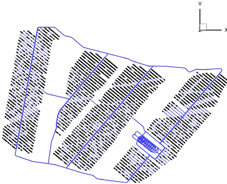
Figure 5-20. Positions of the 5,147 deposition holes that did not pass the \{Q1\} criterion (Variant I).
