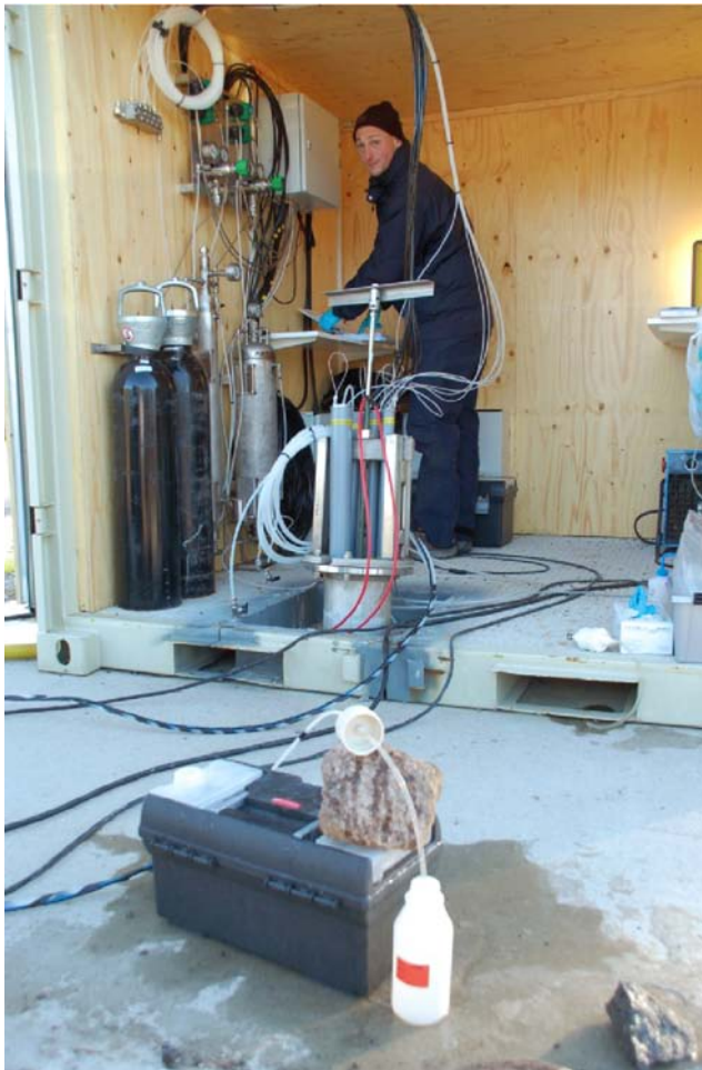
Figure 3-1. Water sampling from a circulation section (the wide stand pipe) in one of the cored drillholes at Laxemar during the monitoring campaign in March 2008.
