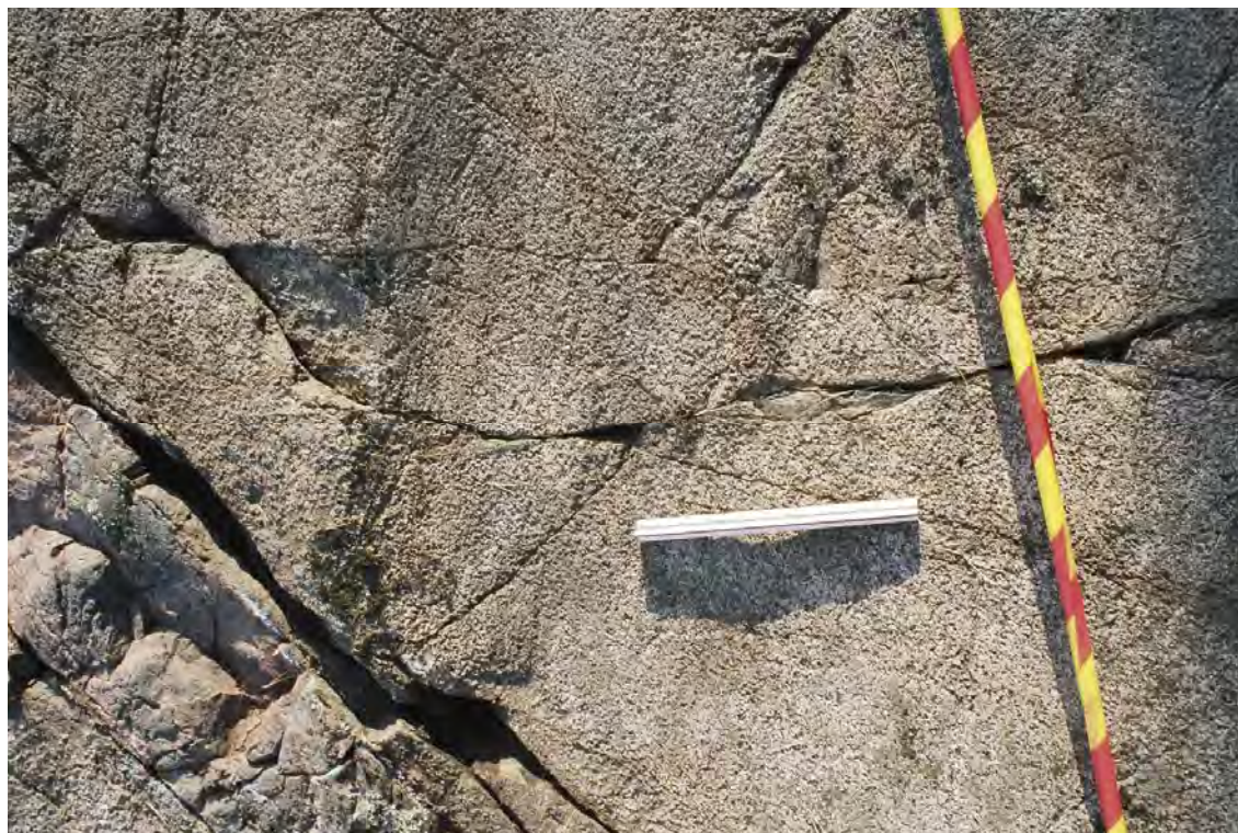
Figure A-5. Photograph from the southern margin of the ASM000206 outcrop, showing the contact between quartz monzodiorite and a granite dyke. Note the secondary red staining along certain fractures. The ruler is 30 cm.
