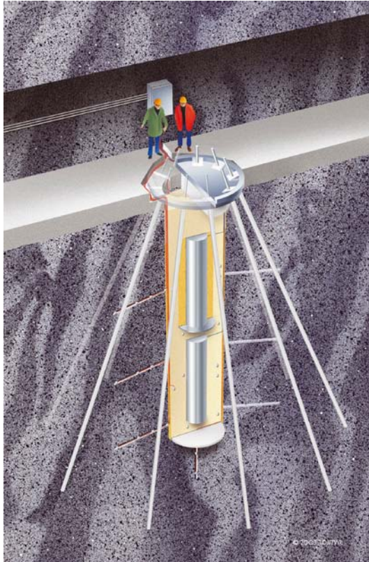
Figure 4-6. The Temperature Buffer Test /after SKB 2005/.
