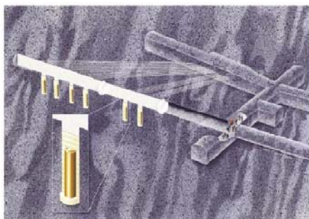
Figure 4-10. The Prototype Repository simulation at Äspö /SKB 2005/.
