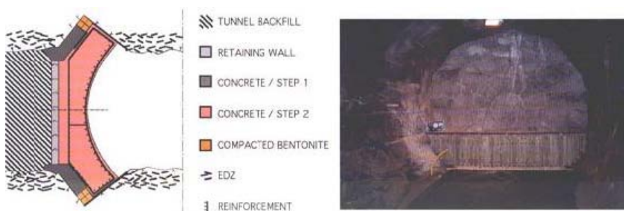
Figure 4-8. The keyed portion of the Backfill and Plug Test and the downstream face of the completed plug /Gunnarsson et al. 2002/.
