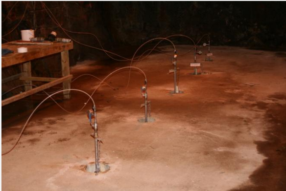
The Taso-tunnel and five boreholes (distance 1.5 m) used for initial characterisation and selection of site.
