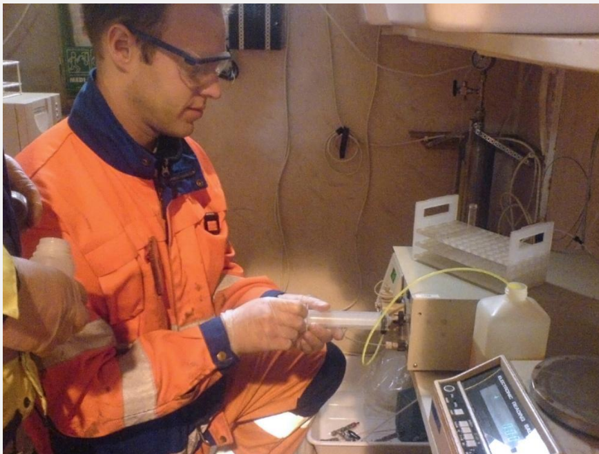
Injection of tracer in fracture.
