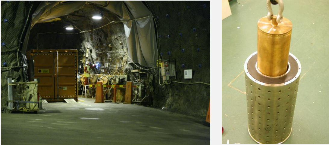
Experimental installation for MiniCan experiment (left) and model canister assembly being lowered into support cage (right).
