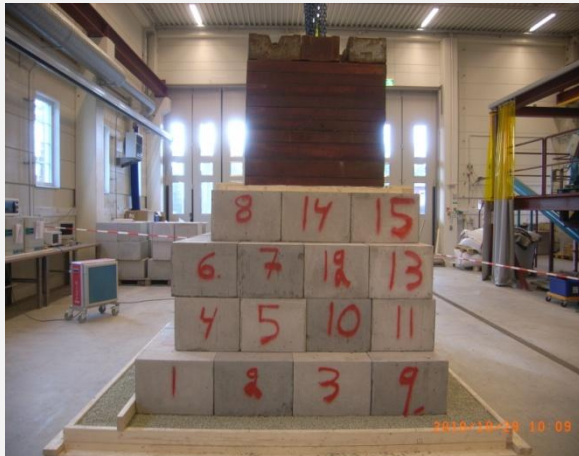
Bottom bed tests in the Bentonite Laboratory.
