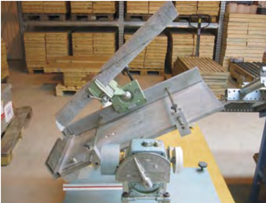
Figure 3-1. NGI's tilt test apparatus.
