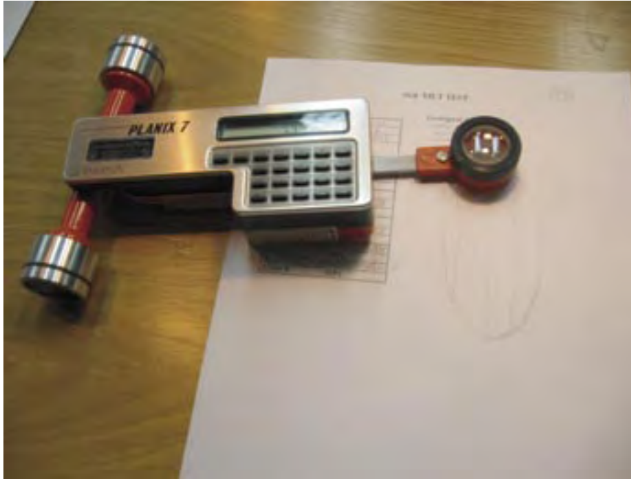
Figure 4-2. Planimeter for measuring the fracture surface area.
