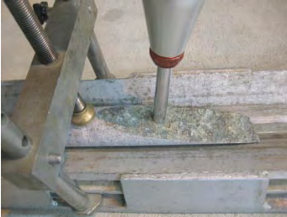
Figure 3-2. Clamp for the Schmidt hammer tests.
