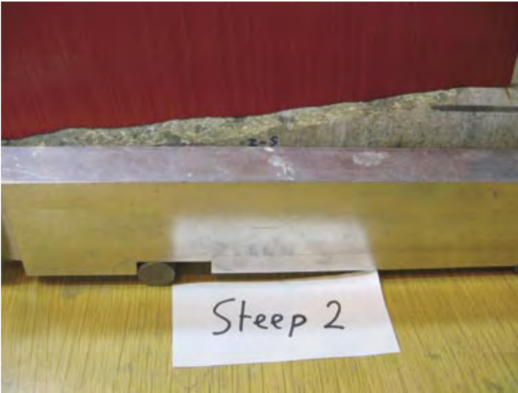
Figure 3-3. Profilometer applied on a joint surface.
