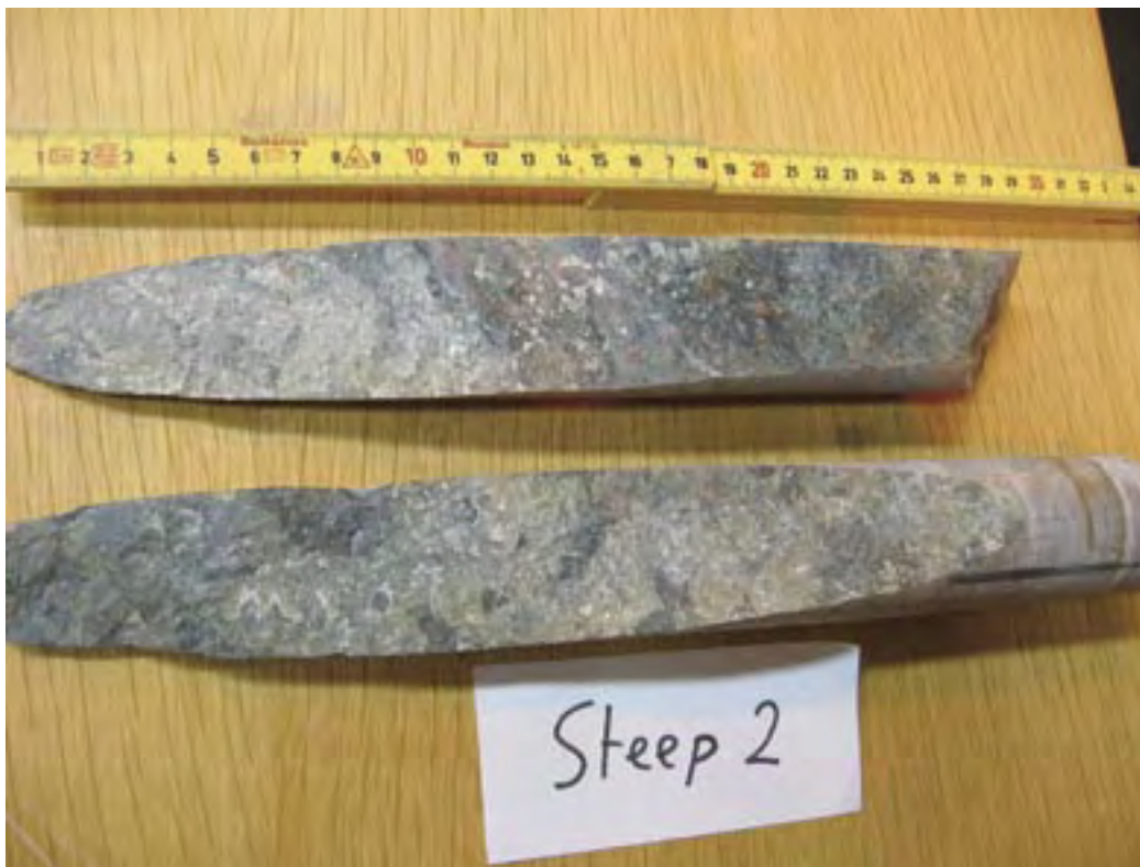
Figure 4-1. Sample for tilt testing in the tilt apparatus.
