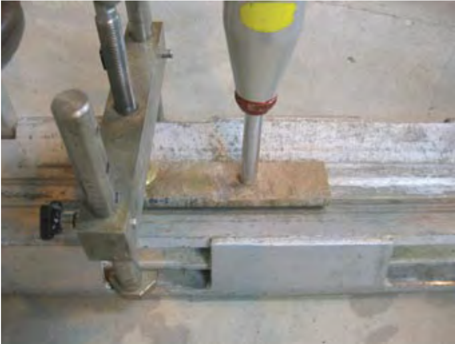
Figure 3-2. Clamp for the Schmidt hammer tests.
