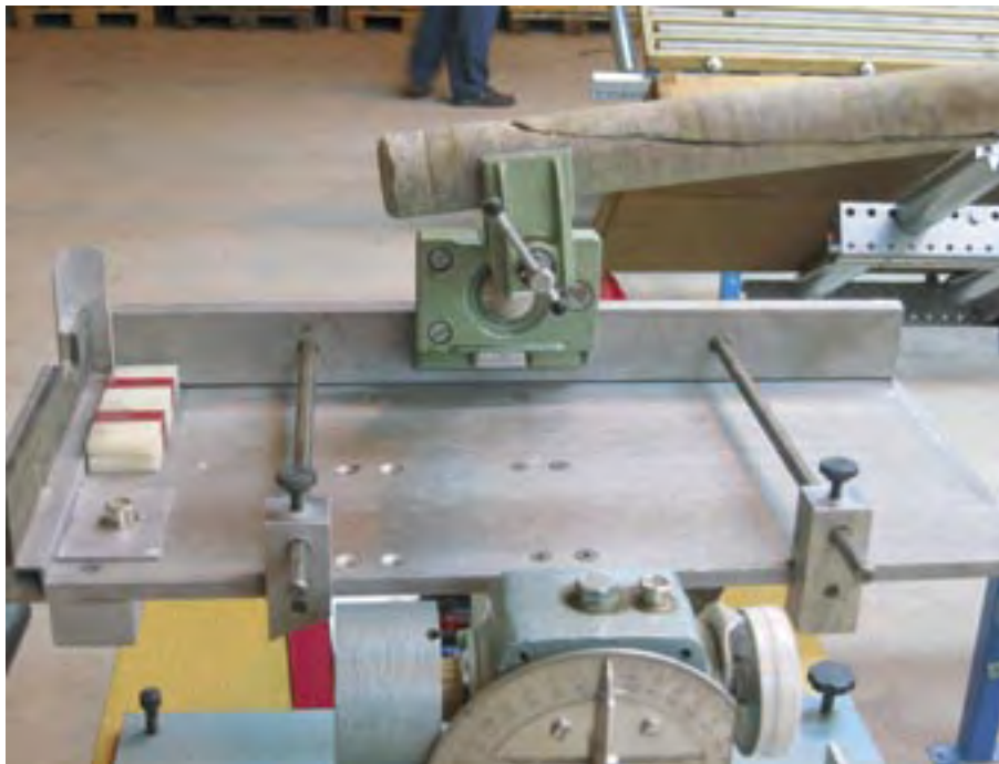
Figure 3-1. NGI's tilt test apparatus.
