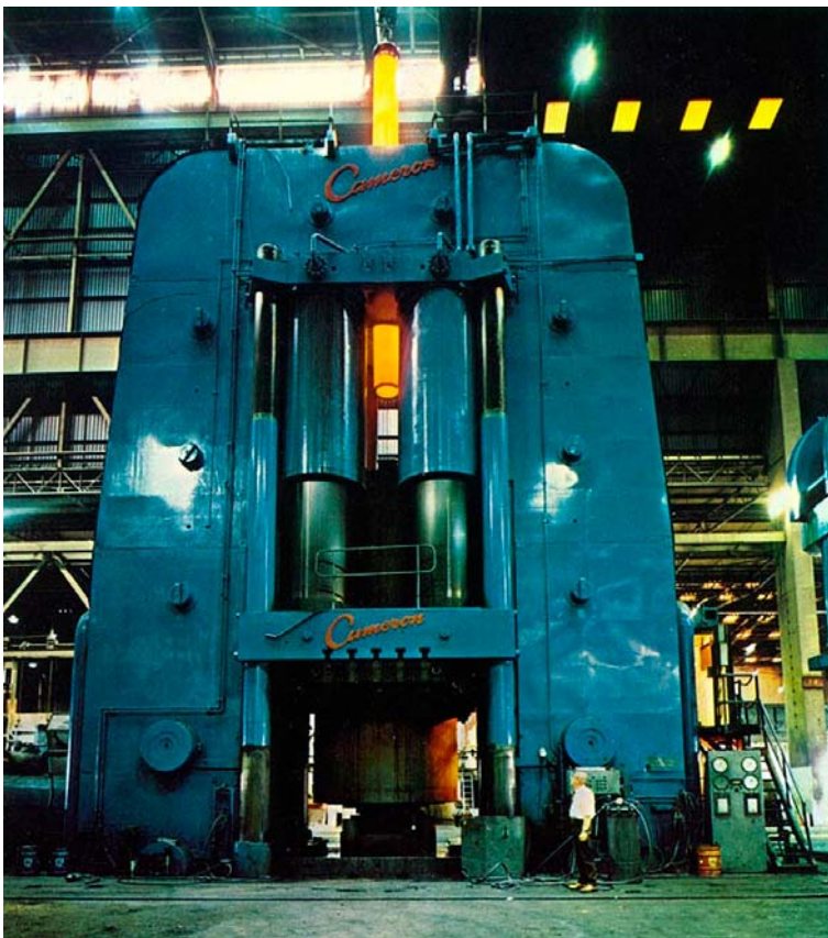
Figure 5-11. The photo shows the extrusion of a tube.
