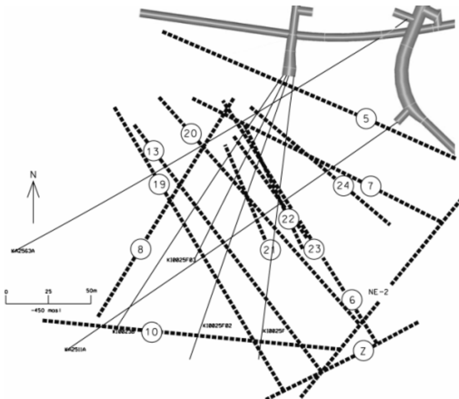
Figure 2-1 Plan view of Äspö TRUE Block Scale site including tracers of boreholes and interpreted structures (Hermanson and Doe, 2000) (Dashed lines represent interpreted deterministic structures, thin solid lines represent boreholes)
