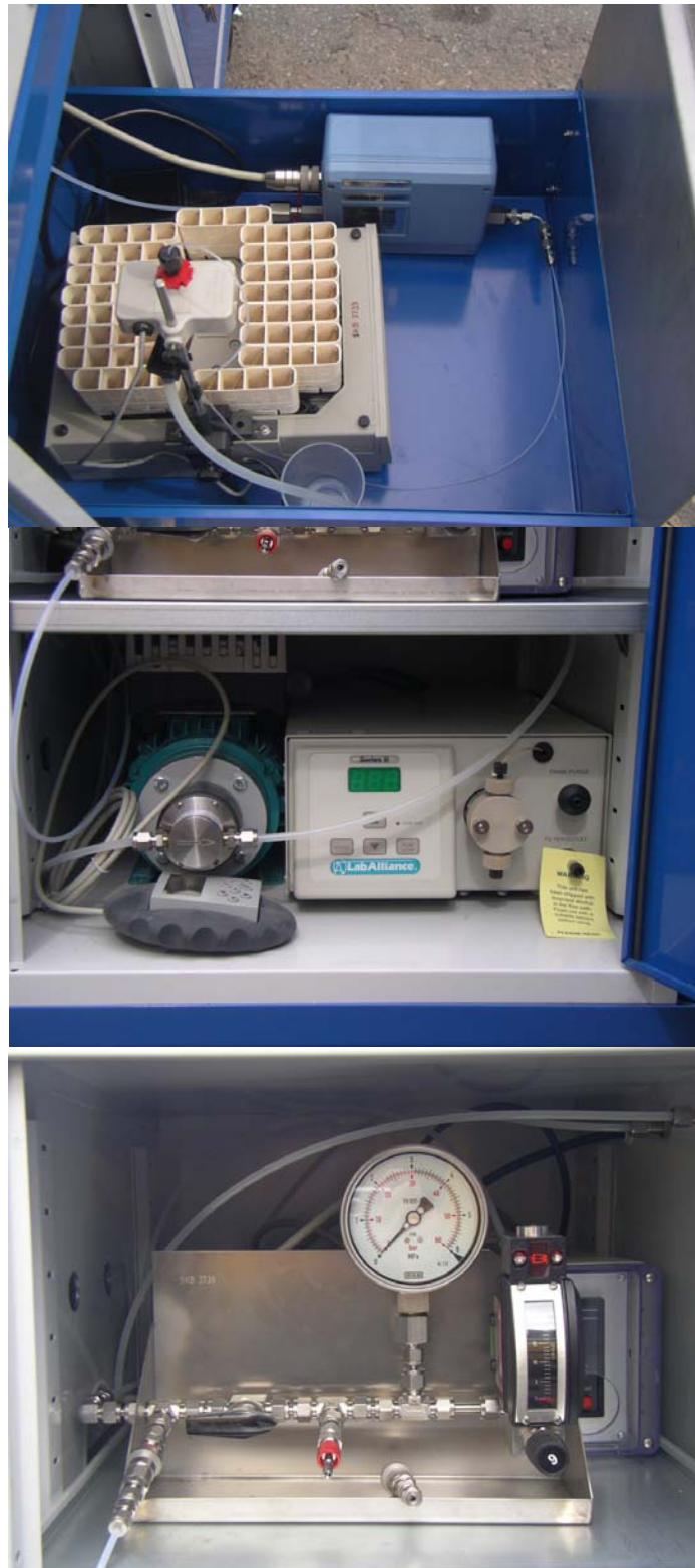
Figure 4-2. Equipment from the dilution test: flow controller and fractional sampler (upper picture), circulation- and injection pump (middle) and the circulation board with flow meter and manometer (lower picture).
