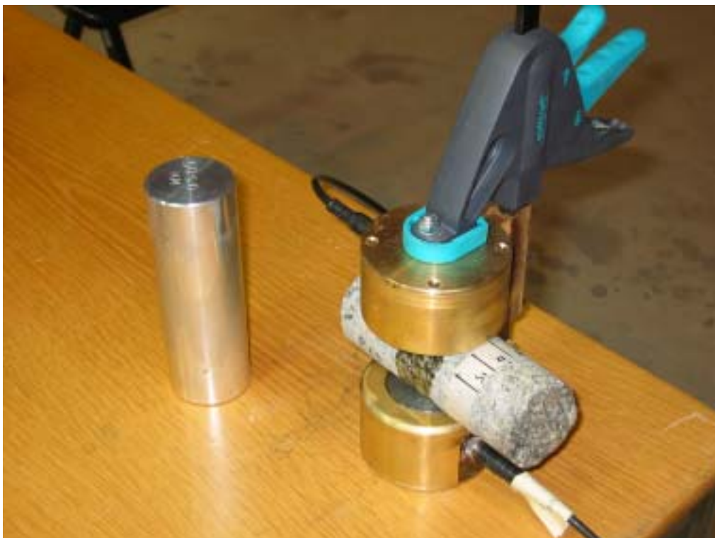
Figure 2-2. Detail of NGI's apparatus for measuring acoustic P-wave travel time transverse borehole core. The aluminium cylinder for calibration of the device is on the left.
