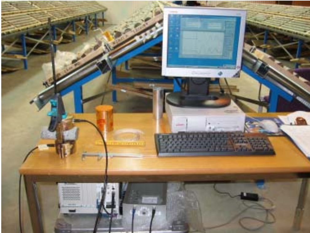
Figure 2-1. NGI's equipment set up for measuring acoustic P-wave travel time transverse borehole core.
