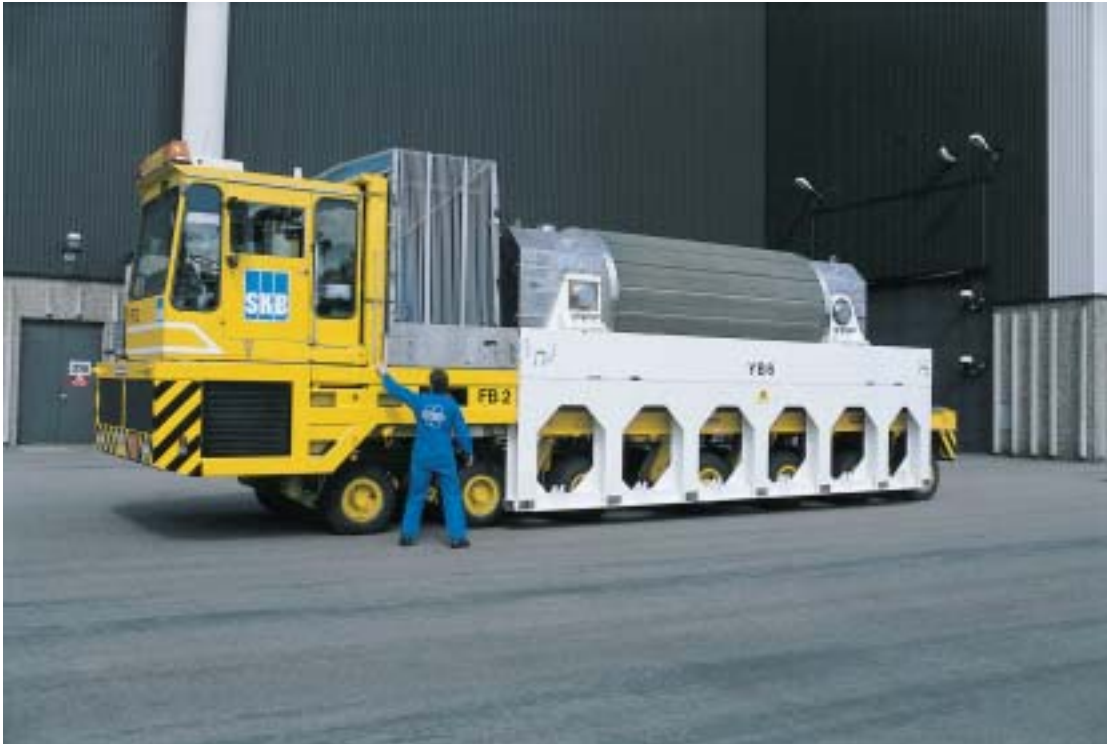
Figure 3-4. Terminal vehicle with fuel transport cask.
