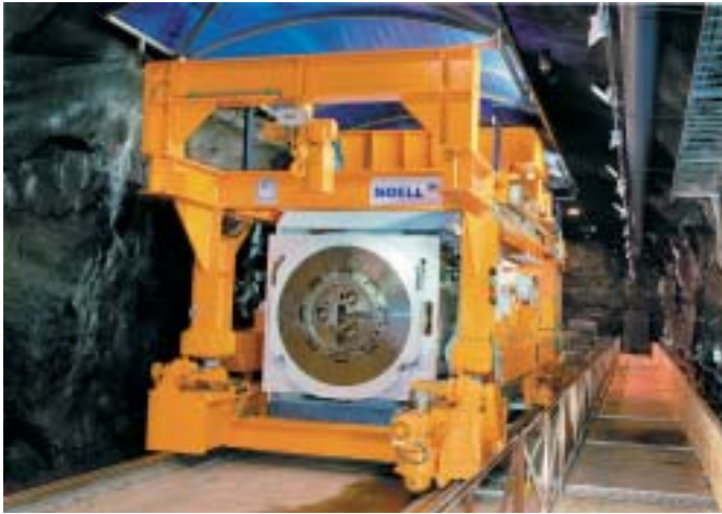
Figure 3-3. Demonstration facility in the Äspö HRL with deployed deposition machine.
