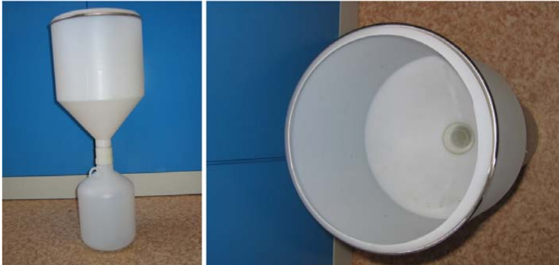
Figure 3-2. The sampler used in summer at the site for sampling of precipitation at the island of Äspö.
