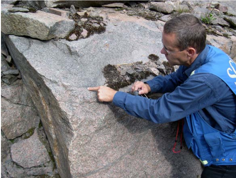
Figure 4-13. Diffuse transition between the red to greyish red, equigranular granite (beneath finger) and the reddish grey, porphyritic Ävrö granite (above finger).
