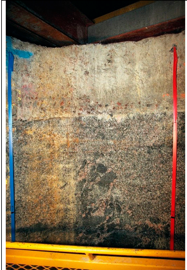
Appendix 11C. Photos from deposition hole DA3147G01 (photos: Lars Andersson, SKB). Upper part of the hole. Boundary between concrete (top) and bedrock below. Rock types: Äspö diorite (greyish) and impure greenstone xenolith (dark grey – black). The blue and red ribbons were used during the mapping procedure not only for orientation but were also a part of a grid system
