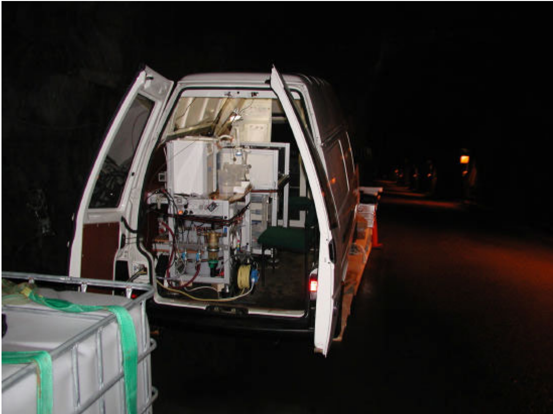
Fig. 6: LIBD instrumentation in the Äspö Hard Rock Laboratory access tunnel
