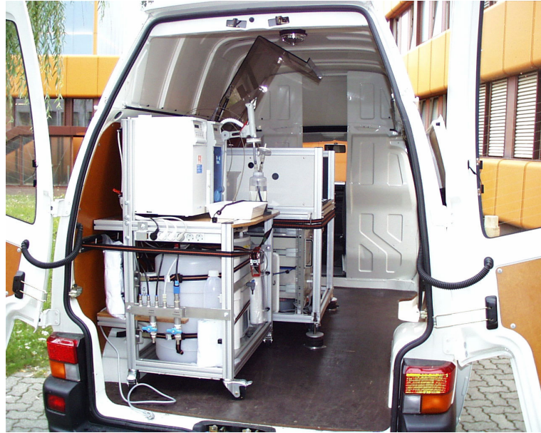
Figure 4: The equipment for Laser-induced Breakdown-Detection (LIBD) of colloids is installed in a van in order to allow mobility and on-line measurements at boreholes (Hauser et al., 2002).
