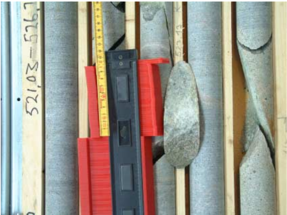
Figure 3-2. Examples of \mathcal{F}_r = 1.5 (or 2.0-) and \mathcal{F}_a = 4 due to clay coating/thin filling.
