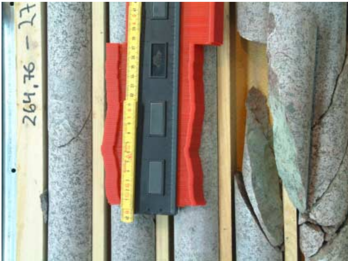
Figure 3-3. a) Examples of \mathcal{J}_r = 1.0 and 1.5. b) Example of \mathcal{J}_r = 3 and \mathcal{J}_a = 4 .
