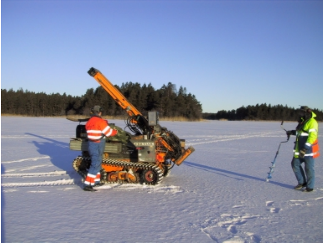
Figure 3-2. The light drilling rig Geotech 604D was used mainly for the drillings performed from the ice-covered lakes.
