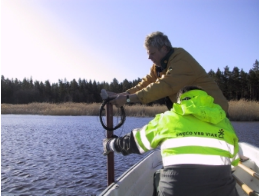
Figure 4-3. Groundwater monitoring well SFM0012 placed in the sediments below open water.
