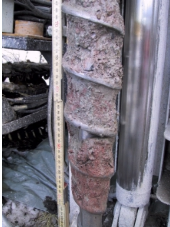
Figure 4-1. Soil sampling by auger drilling.
