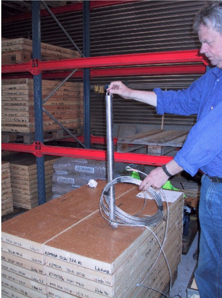
Figure 4-1. The stainless-steel slug that was used to create the water-level displacement in all 2-inch observation wells. The length of the slug can be adjusted by adding or removing 0.25- and 0.50-m sections.
