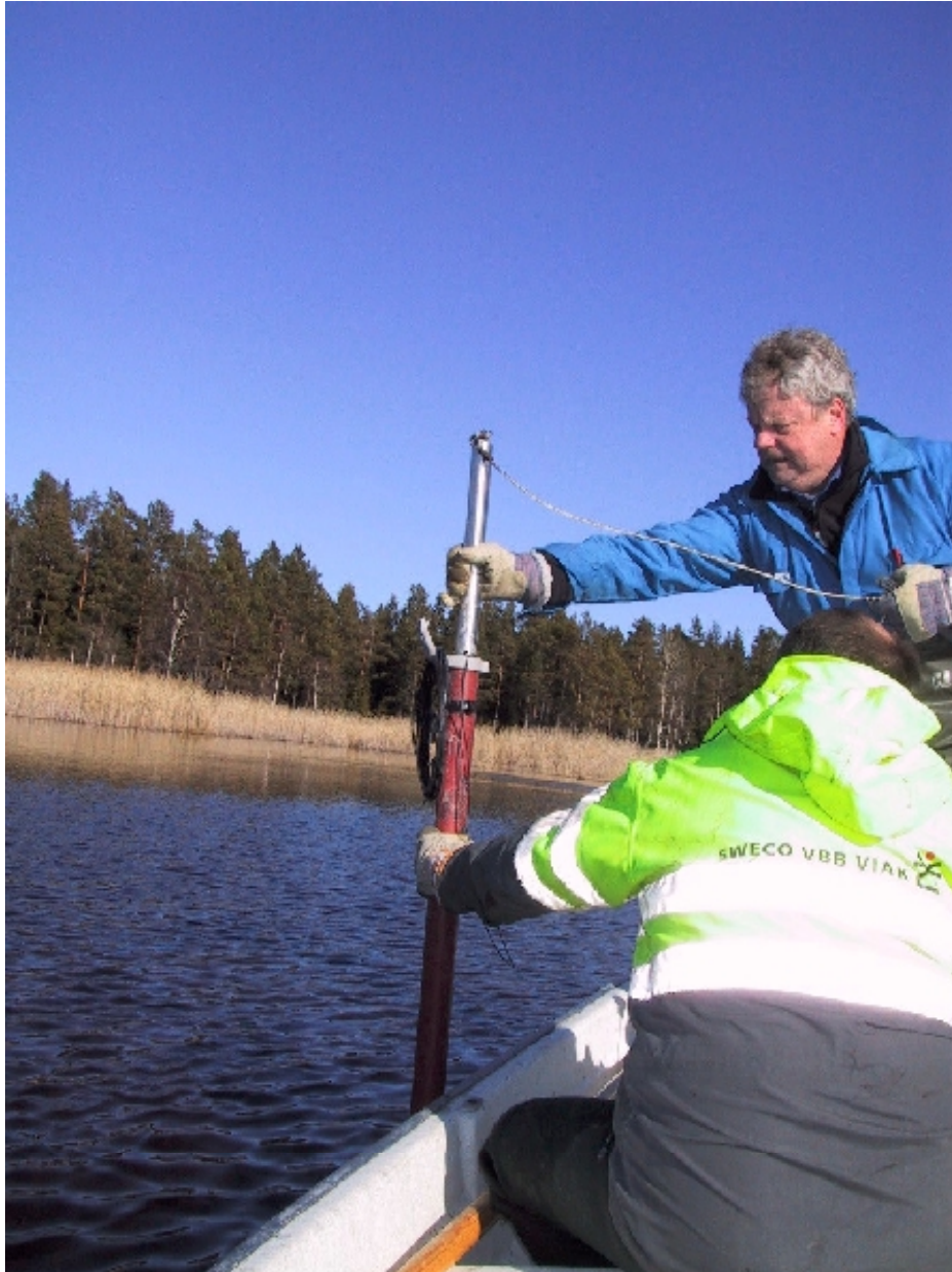
Figure 5-1. Initiation of falling-head test in groundwater monitoring well SFM0012. One of the operators is holding the slug connected to the wire, and the black cable connected to the Diver® (already lowered into the well) is hanging on top of the well. After trying out different types of wire stops, it was found that a spanner wrench was most suited for this purpose. For security reasons, two persons had to perform the slug tests in wells installed in soil below open water.
