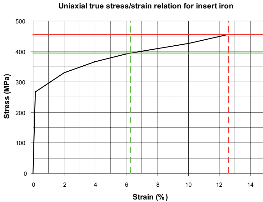
Figure 3-1. The ultimate strength is 456 MPa (red lines) and the corresponding strain is 12.6% with the reliability of 90% according to the material testing. The maximum allowable effective (von Mises) stress (green lines) is set in a way that the respective strain is half of the strain ( A_3 ) corresponding to the ultimate tensile strength (UTS=456 MPa). The green lines are at 6.3% and 395 MPa. The basic curve is the average tension test results (true stress) in 20°C with standard test (no strain-rated).
