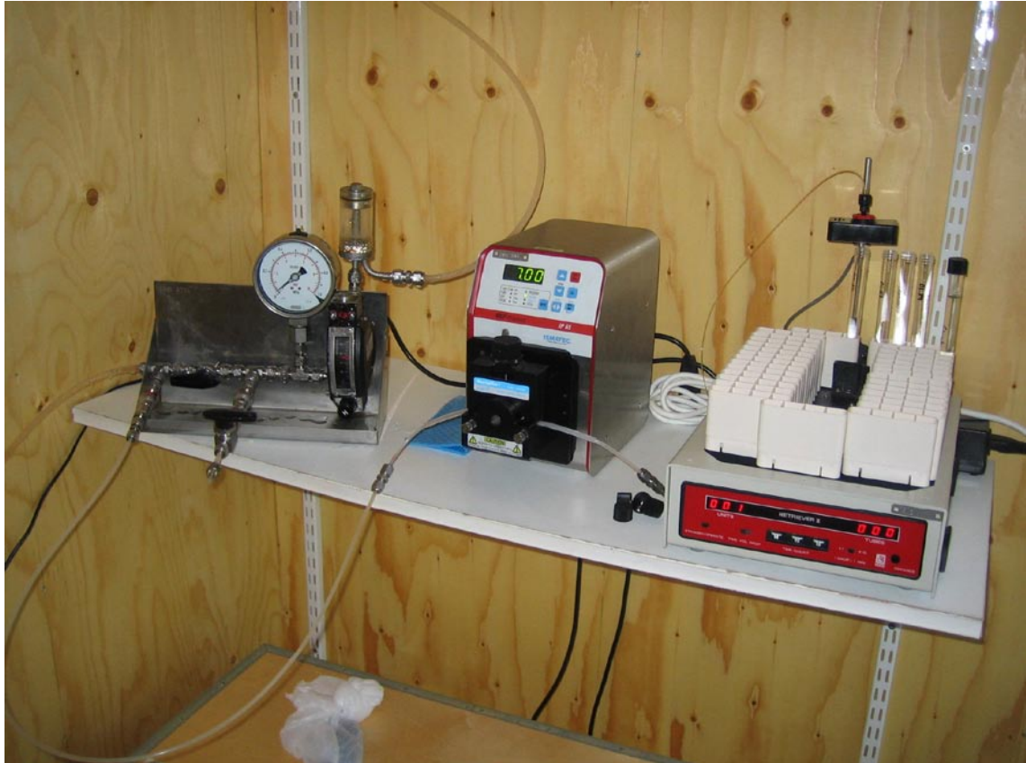
Figure 3-3. Circulation unit, peristaltic pump and fractional sampler used for the groundwater flow measurements and the tracer test.
