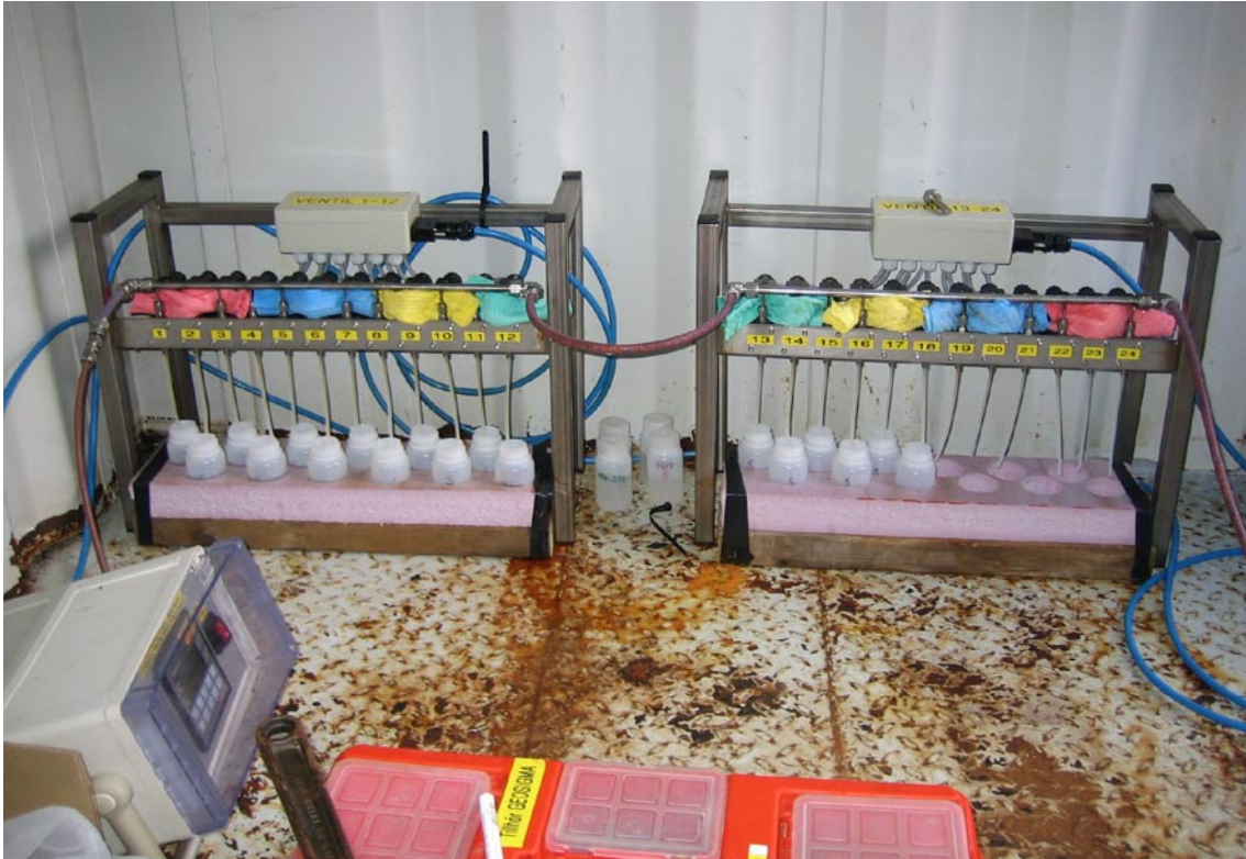
Figure 3-6. The automatic sampling equipment (24 magnetic valves) at the withdrawal borehole HLX28.
