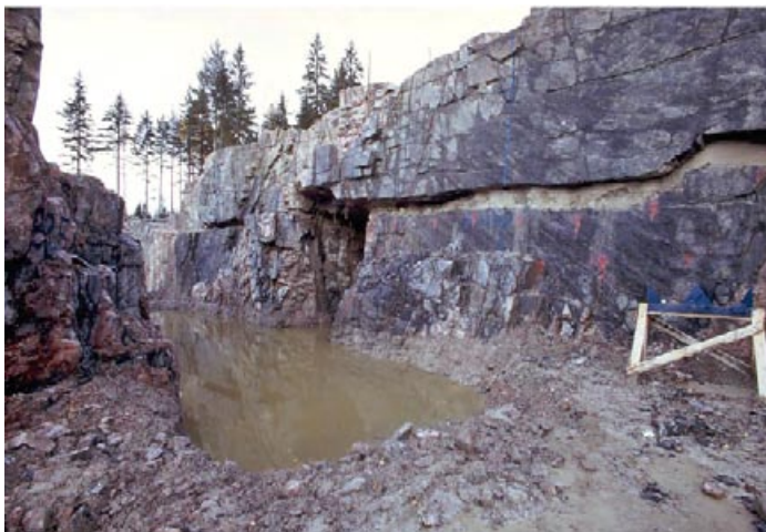
Figure 1-3. Example of a horizontal sediment-filled fracture, which was exposed at Forsmark during the construction of the nuclear power plant in the 1970s, from /Leijon 2005/.
