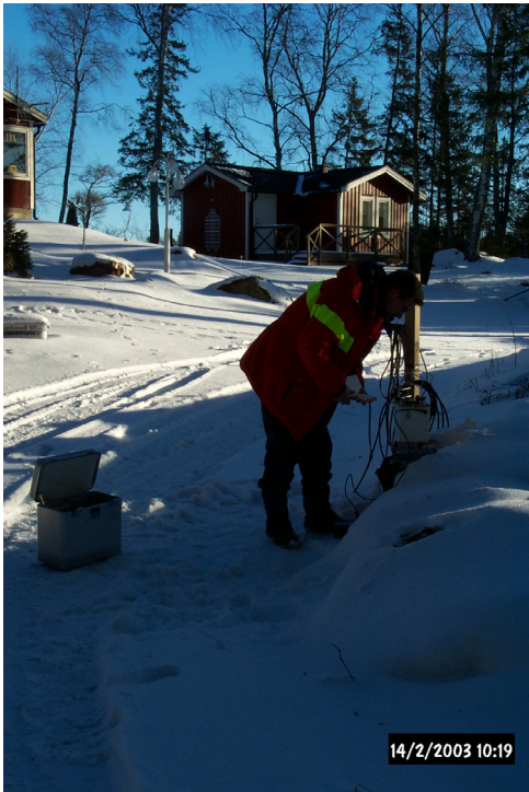
Figure 4-2c. Local base-point UPP39602, in the south-eastern part of the nature reserve Kallrigafjärden. Map-sheet 12I Östhammar. The base-point is connected to RG82 using point “Östhammar A” with the g-value 981908.210 mGal /Haller and Ekman, 1988/. Two connections were made with the gravity meter in damped mode. The difference in the g-value was 0.03 mGal. This base-point was mostly used for the measurements on ice inside and north-east of the reserve.
