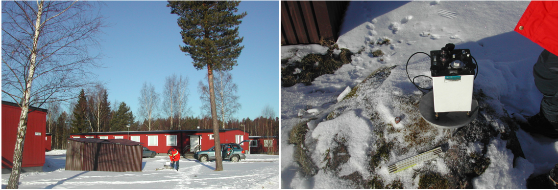
Figure 4-2b. The local base-point UPP39601, 1 km south of the reactors 1 and 2 at Forsmark. Map-sheet 12I Östhammar. The base-point is connected to RG82 using point “Östhammar A” with the g-value 981908.210 mGal /Haller and Ekman, 1988/. Two connections were made with the gravity meter in damped mode. The difference in the g-value was 0.04 mGal.
