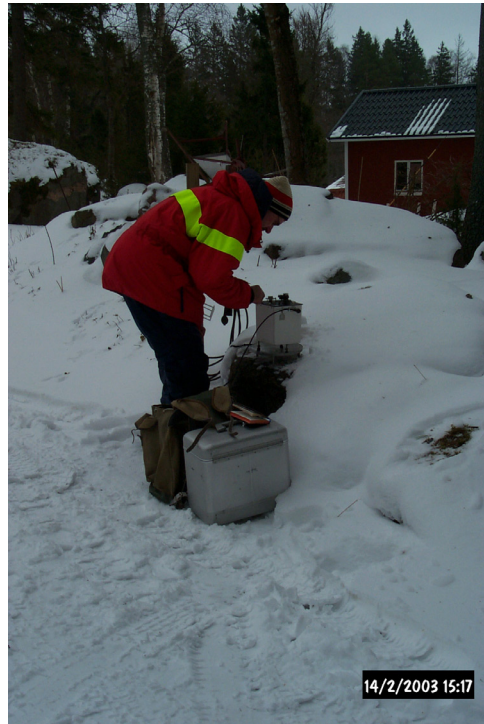
Figure 4-2c. Local base-point UPP39602, in the south-eastern part of the nature reserve Kallrigafjärden. Map-sheet 12I Östhammar. The base-point is connected to RG82 using point “Östhammar A” with the g-value 981908.210 mGal /Haller and Ekman, 1988/. Two connections were made with the gravity meter in damped mode. The difference in the g-value was 0.03 mGal. This base-point was mostly used for the measurements on ice inside and north-east of the reserve.
