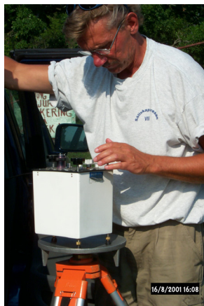
Figure 3-1. Measurements with LaCoste & Romberg land gravity meter.
