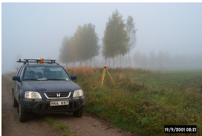
Figure 3-2. High precision GPS-system used by SGU. The receiver with the antenna on the tripod is used as the reference station and the receiver in the car as a rover. The antenna for the rover is situated on the roof of the car.
