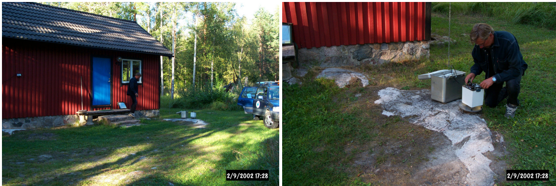
Figure 4-2a. The local base-point UPP18501, Lill Vamsta, on map-sheet 12I Östhammar. The base-point is connected to RG82 using point “Östhammar A” with the g-value 981908.210 mGal /Haller and Ekman, 1988/. Two connections were made giving very small difference in the g-value, below 0.01 mGal.
