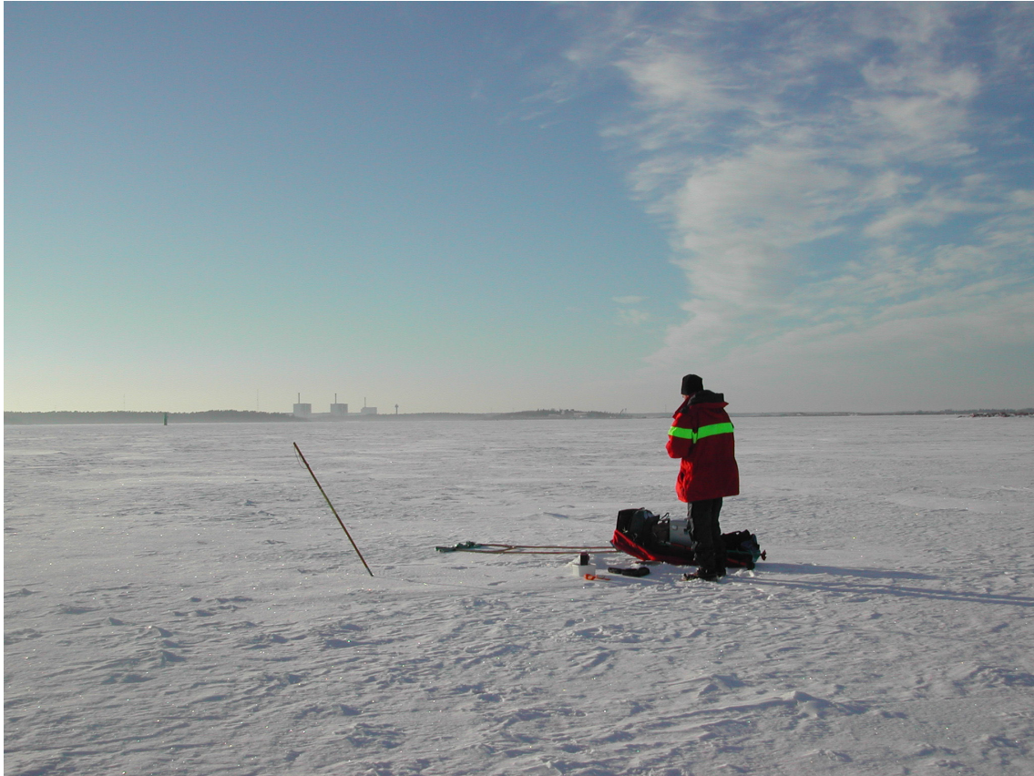
Figure 4-1b. Gravity measurements on ice in the strait Öresundsgrepen. The ice thickness was approximately 40 cm. This is sufficient for good quality measurements during calm days.
