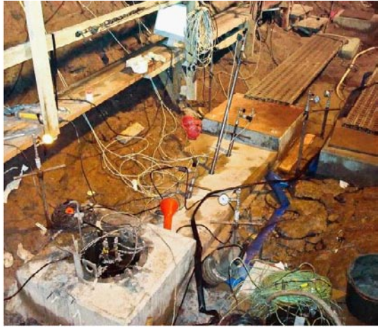
Figure V-17. Shows the injection holes with installed packers during the hydraulic testing of the damaged zone in KQ0046G03.
