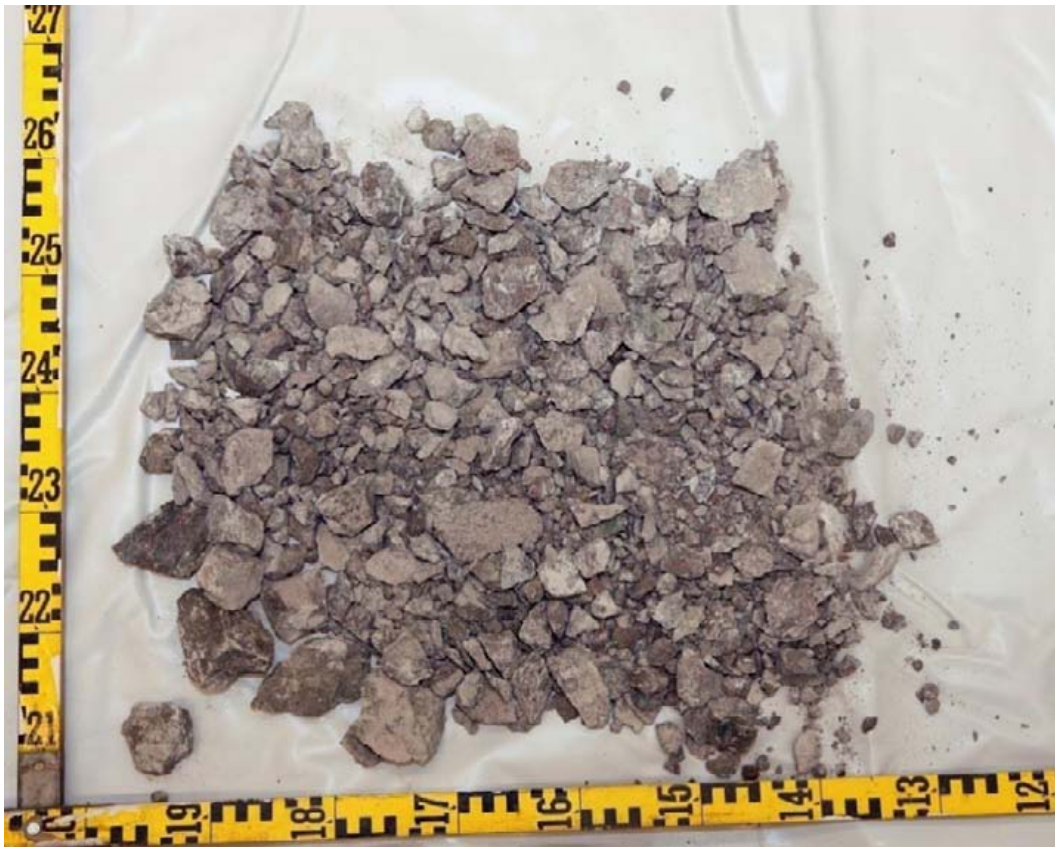
Figure AL2-6. Collected fragments from the bottom in heating hole KQ0048G04 by the suction pipe (Test 3).
