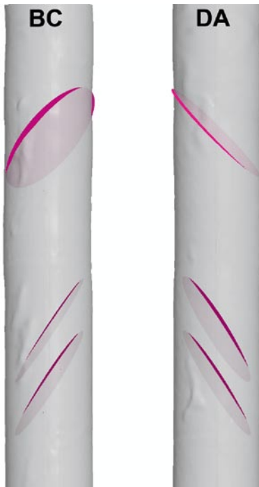
Figure S-10. Mesh from the laser scanning in KQ0051G05 showing the spalling and the shear zone in the hole. Discs mark the upper and lower boundary of the zone and the internal foliation. The spalling is not very pronounced in the borehole and is mostly absent within the strongly sheared parts of the shear zone.
