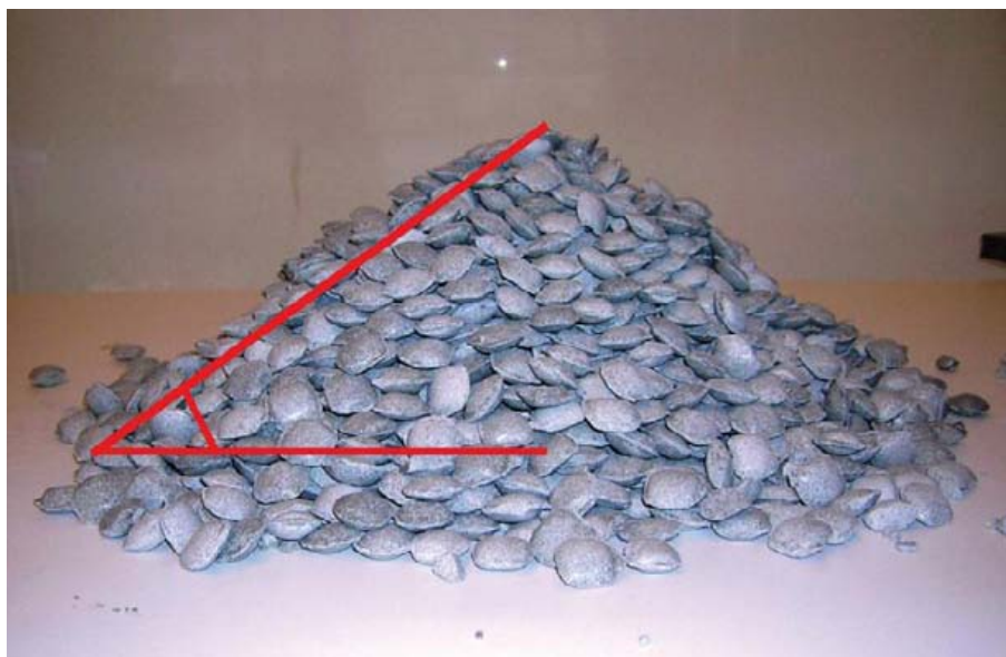
Figure F-1. Picture showing a heap of MX-80 pellets. The red angle shows how the angle of friction was determined.
