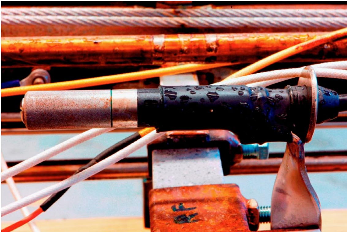
Figure 3-7. Close-up view of the type of RH-gauges (Rotronic) used temporarily in the late part of initial field test and for continuous readings in the second field test (Photo C-R Lindqvist).
