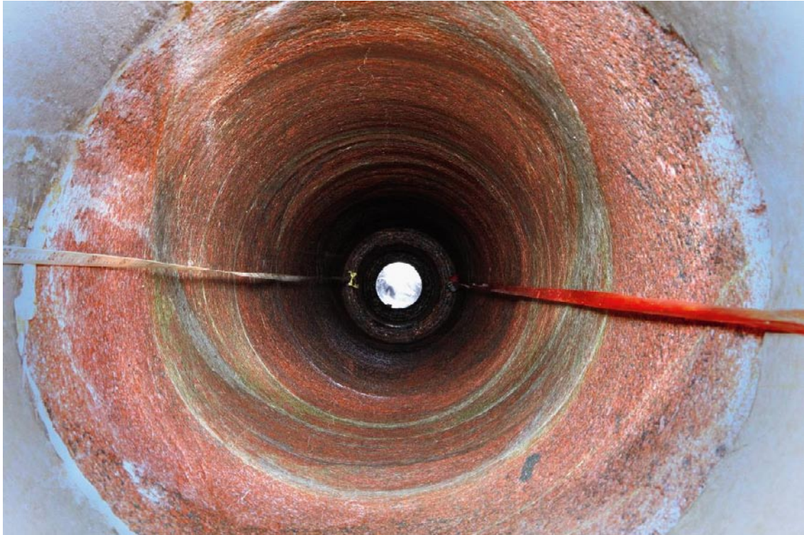
Figure T-15. Photograph of borehole KQ0046G04 in Field Test 4 before initiating the heating phase.
