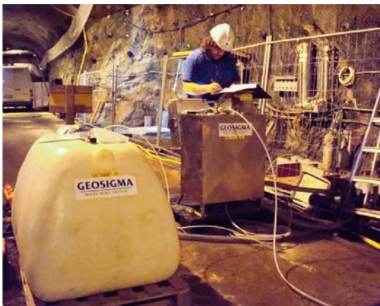
Figure V-16. Shows the equipment utilized for the water injection tests of the damage zone in KQ0046G03.
