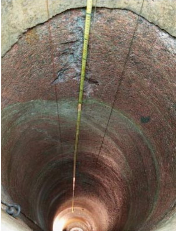
Figure T-32. Photographs of the borehole wall in heating hole KQ0046G04 after scaling the wall from loose rock fragments. Field Test 4 was performed with confinement.
