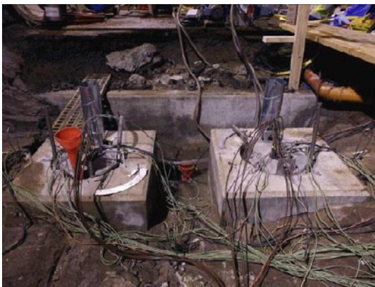
Figure V-12. Shows the test equipment in place after filling the slot with pellets in the preparation for Field Test 4.
