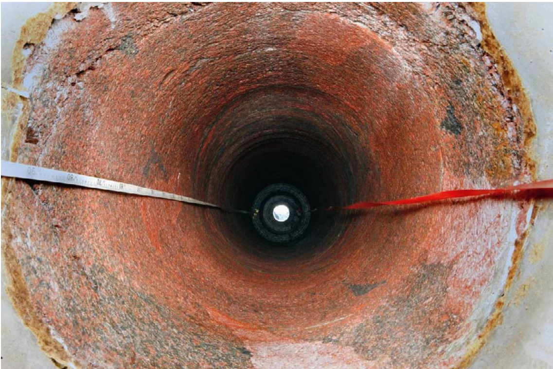
Figure T-6. Photograph of borehole KQ0051G05 in Field Test 2 before initiating the heating phase.
