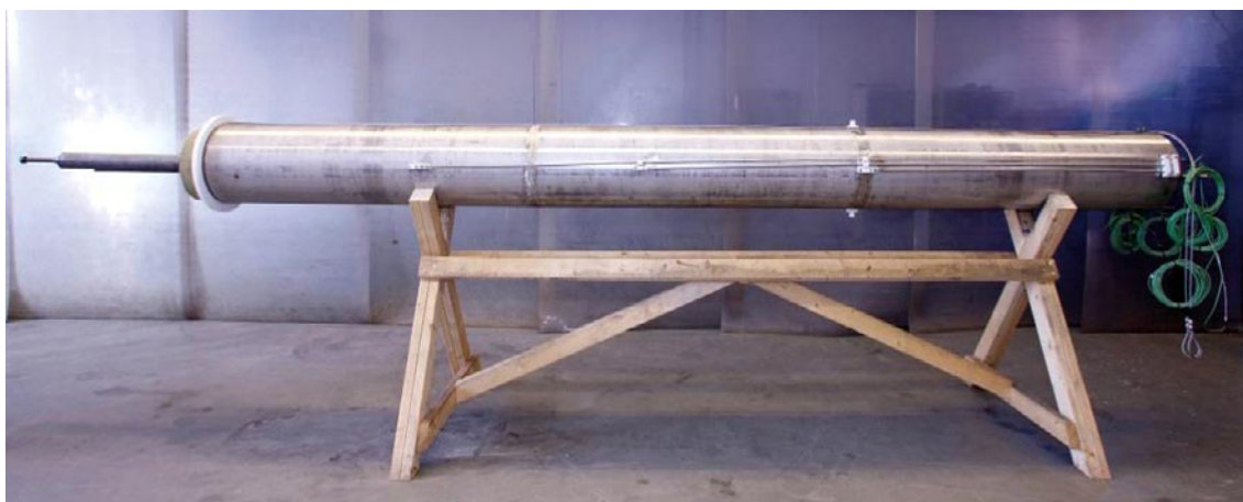
Figure U-3. Shows the instrument holder installed in Field Test 3.
