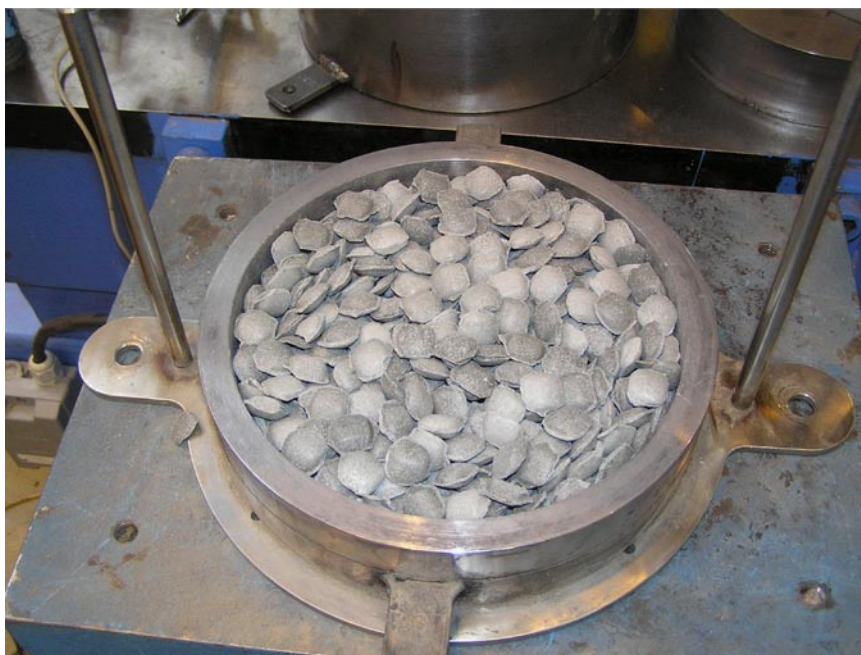
Figure E-2. The bentonite material placed in cell.
