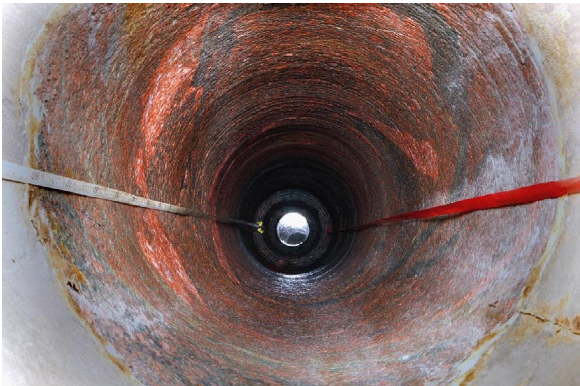
Figure T-2. Photograph of borehole KQ0054G04 in Field Test 1 before initiating the heating phase.
