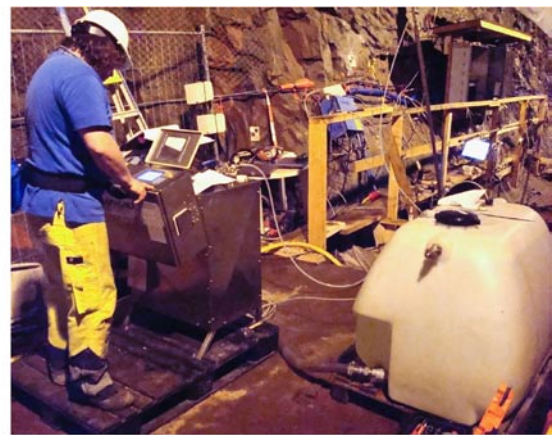
Figure V-16. Shows the equipment utilized for the water injection tests of the damage zone in KQ0046G03.
