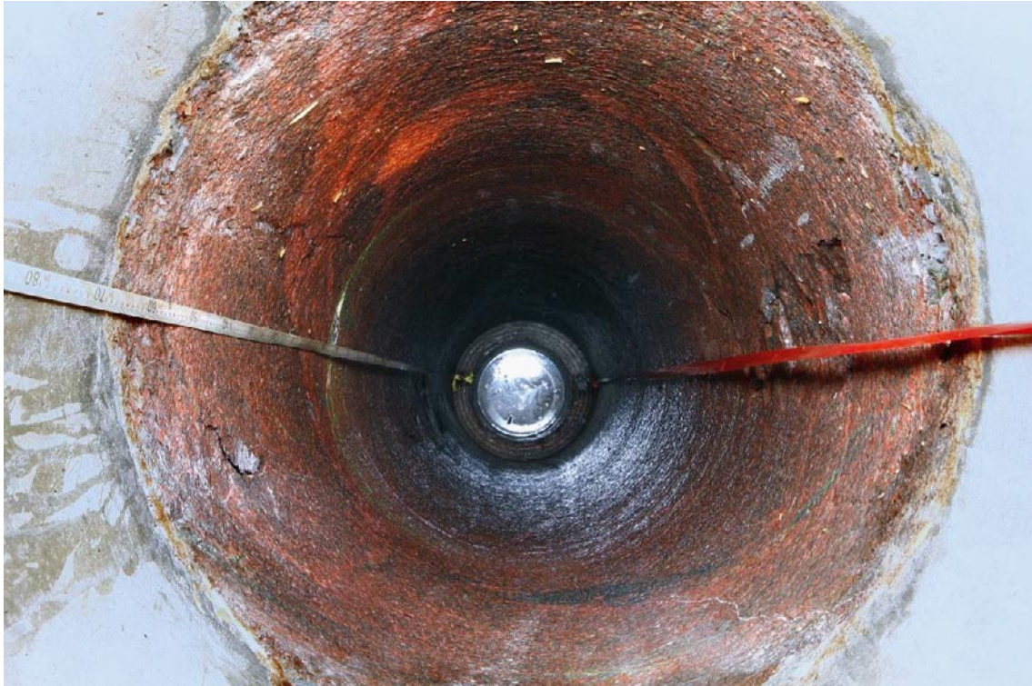
Figure T-7. Photograph of borehole KQ0048G04 in Field Test 3 before initiating the heating phase.
