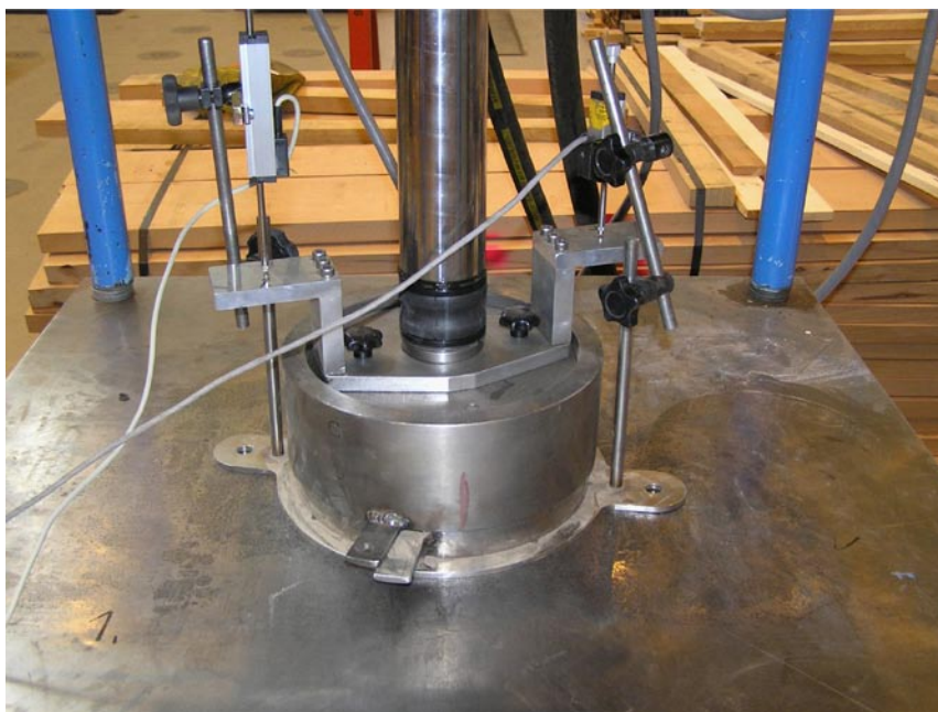
Figure E-4. The oedometer cell is placed in the load frame. The piston is pressing on the cell cover via a spherical joint. The two linear displacement transducers are installed.
