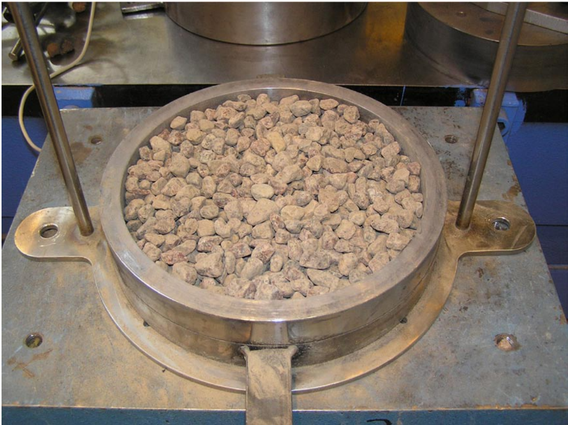
Figure AE-3. The natural gravel is placed in cell.
