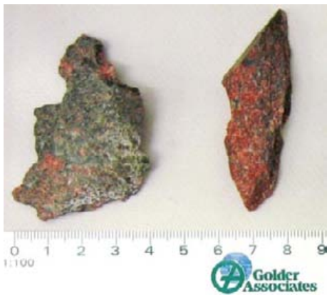
Figure ALI-12. Investigated fragments in heating hole KQ0048G05 (Test 3), Group 1. Fragments that were brought up with a suction pipe.
