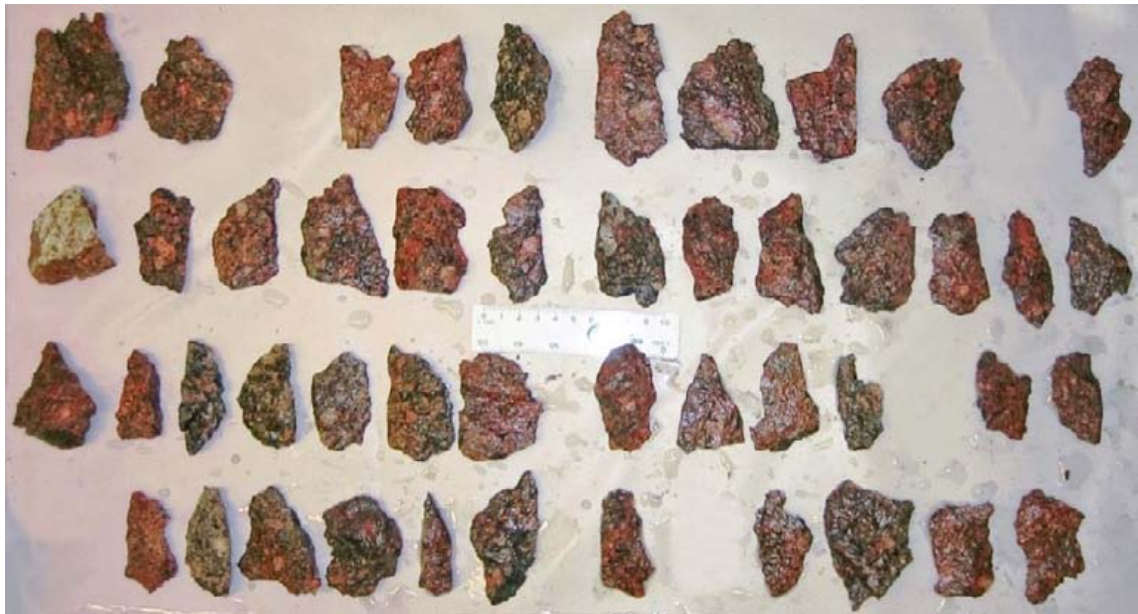
Figure L-2. Photograph of fragments no. 38–89 from hole KQ0048G04. The scale bar is 10 cm.
