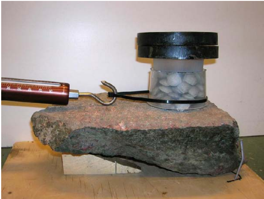
Figure F-2. Principle of the measurements. The picture shows a test where the friction between pellets and a TBM drilled rock surface is tested. The cylinder is filled with MX-80 pellets and a normal force of about 20 N is applied on the top.
