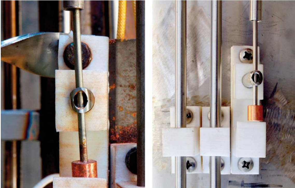
Figure U-6. Shows a close-up view of the spring loaded mechanism after modification before Field Test 2. The edge of the guide bushing has been chamfered.
