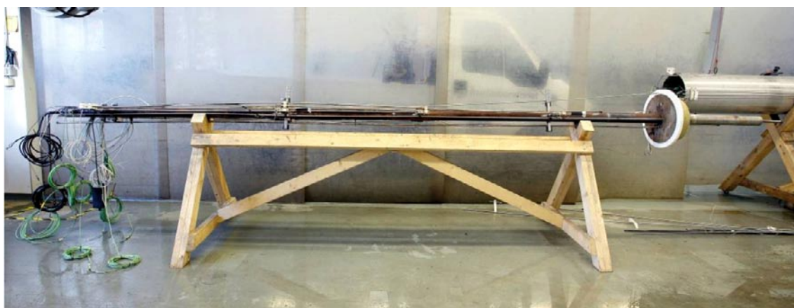
Figure U-2. Shows the instrument holder installed in Field Test 2.
