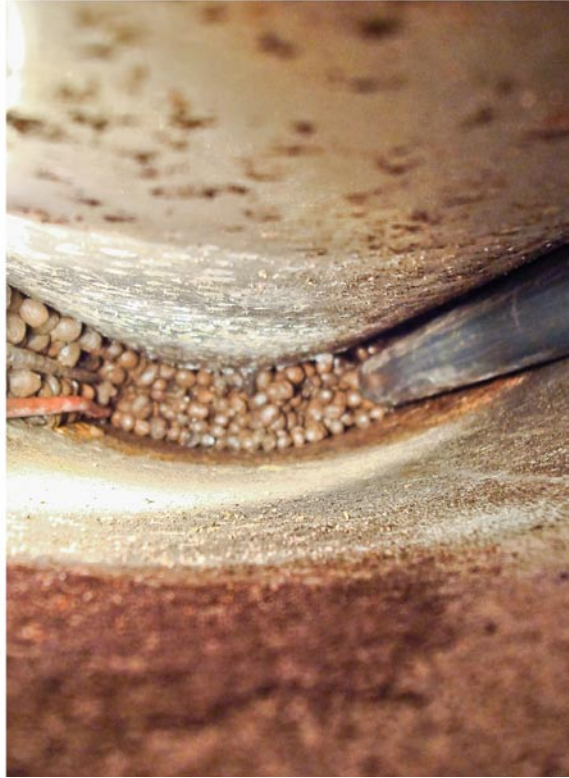
Figure V-9. Shows the emptying of the pellet filled slot after the completion of Test 3.
