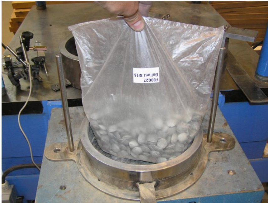
Figure E-1. Bentonite is poured into the cell. (The label on the plastic bag is not correct.)
