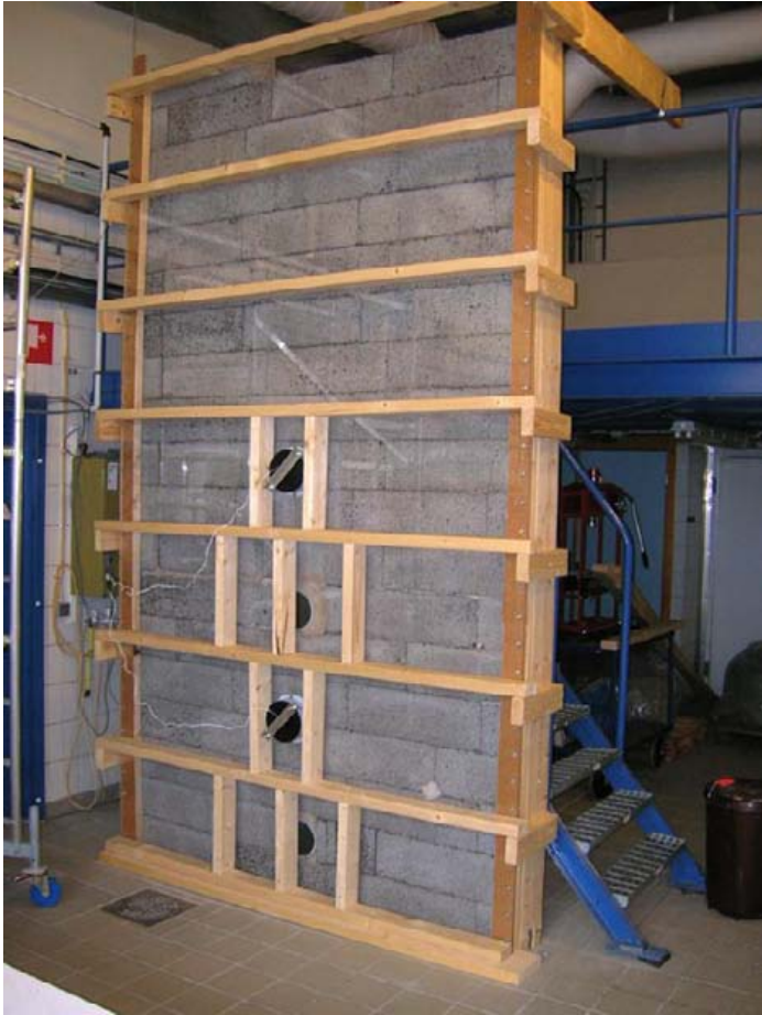
Figure F-6. An artificial slot was built in the laboratory (width=2 m and height 3.6 m). The rock wall is simulated with LECA blocks and the bentonite blocks with Plexiglas. The horizontal pressure can be measured at four points, two on the rock wall and two on the bentonite side.
