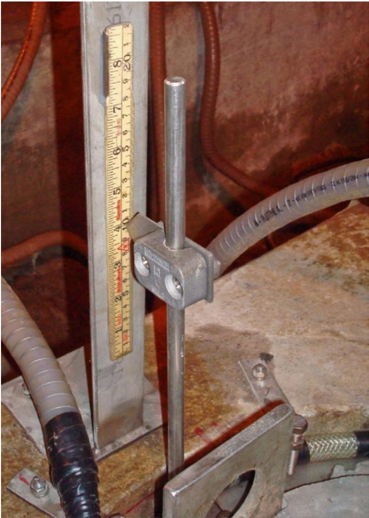
Figure 5-5. Photograph of the level gauge installed in the final heating test for checking movements in the pellet filled slot (Photo R Glamheden).
