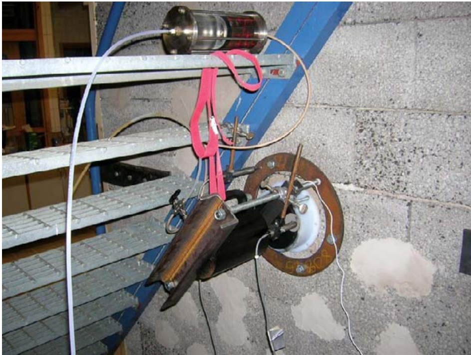
Figure F-12. One of the pressure cells on the “rock” side was rebuilt and equipped with a hydraulic piston which was controlled by a GDS (microprocessor controlled pump). This made it possible to move the piston with a constant rate forward and measure the displacement and the achieved pressure.
