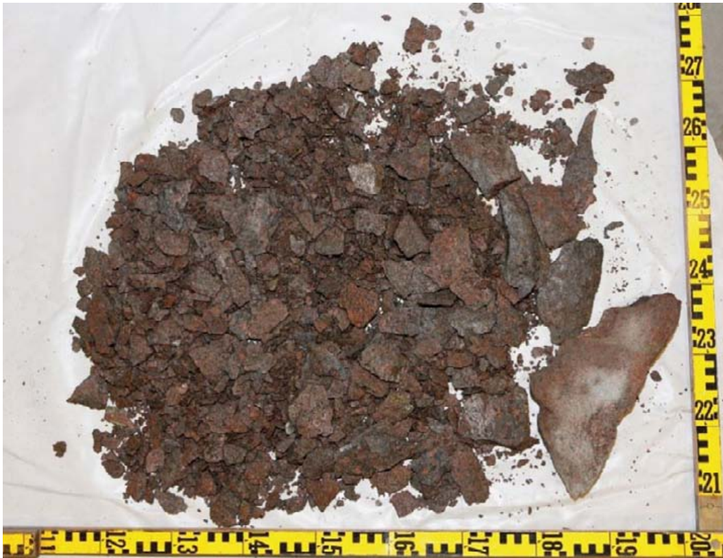
Figure AL2-5. Collected fragments in heating hole KQ0048G04 in Test 3.
