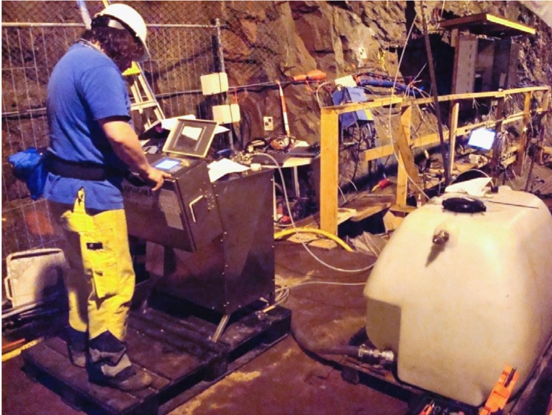
Figure 7-10. Shows the equipment utilized for the water injection tests (Photo R Glamheden).
