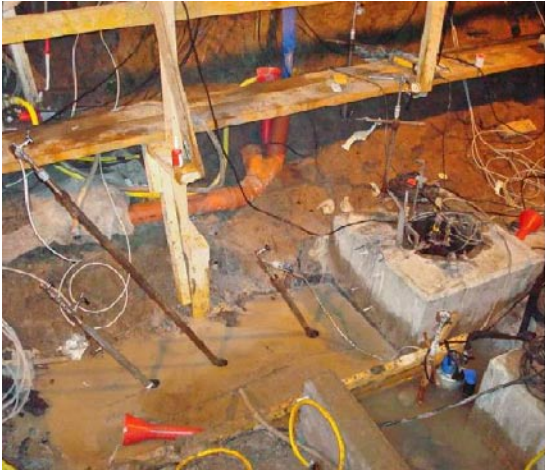
Figure V-17. Shows the injection holes with installed packers during the hydraulic testing of the damaged zone in KQ0046G03.
