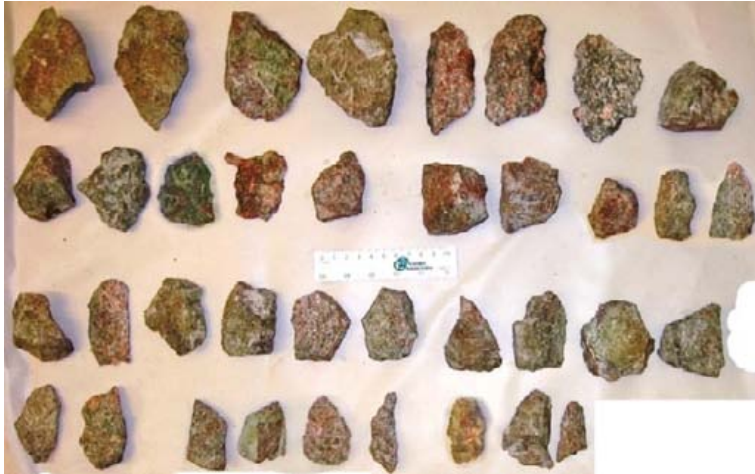
Figure ALI-9. Investigated fragments in heating hole KQ0048G04 (Test 3), Group 1. Fragments that were brought up with a suction pipe.
