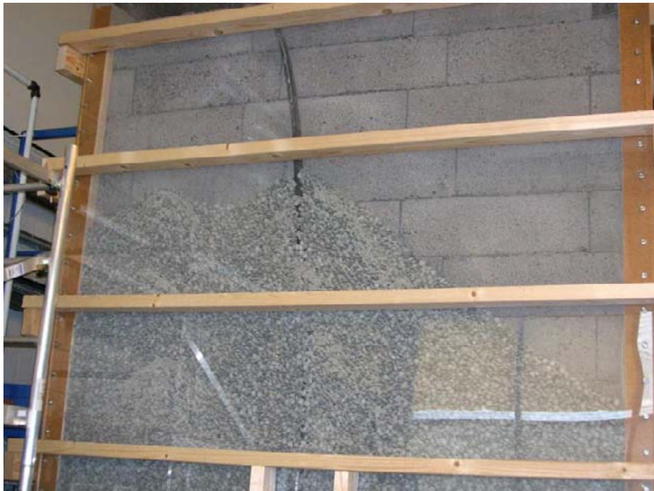
Figure F-9. Photo showing the pellets filling and the tube that holds the vibrating staff inside the pellets filling.
