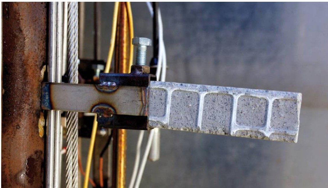
Figure U-5. Shows a close-up view of the spacers in clinker used in Field Test 2.
