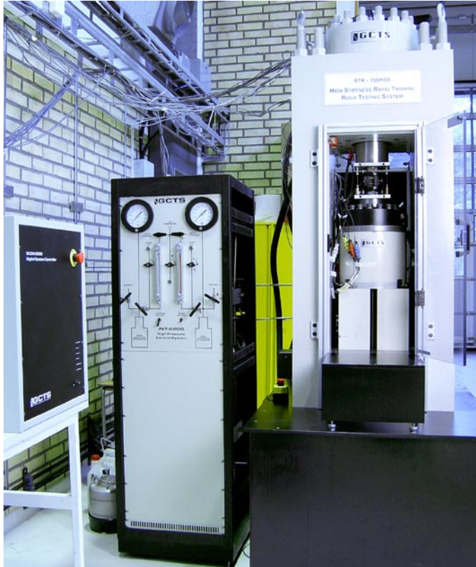
Figure C-1. Rock testing system. From left: Digital controller unit, pressure cabinet (used for triaxial tests) and load frame. The PC with the test software (not shown in the picture) is placed on the left hand side of the controller unit.
