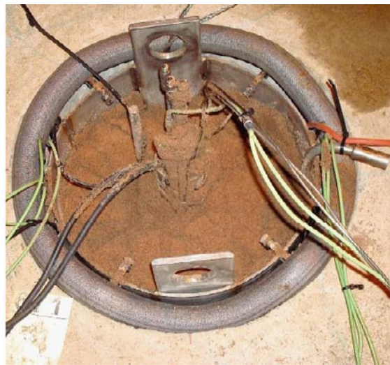
Figure V-6. Shows the test equipment in place before and after sand filling of the larger tube during preparation for Field Test 3.
