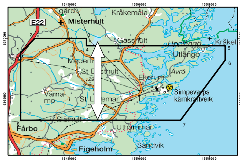
Figure 1-1. Area covered by geophysical measurements from helicopter. Measurement was performed along north-south lines with tie-lines flown east-west.
