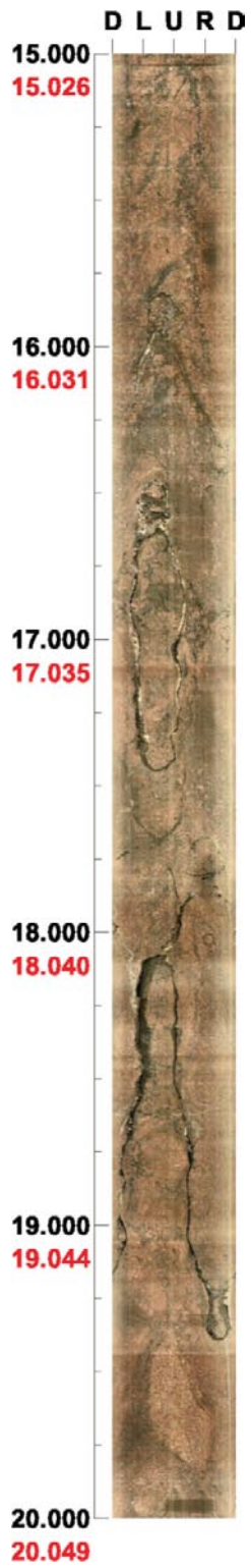
Figure 6-1. BIPS image showing the vertical fracture zone 16.4 m–19.4 m.
