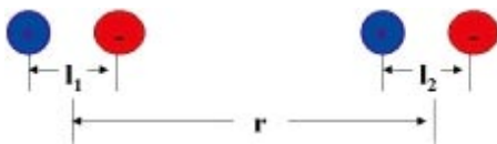
Figure 2-1. A linear arrangement of two dipoles, used to define the potential energy in the Schrödinger equation for the London interaction energy.
