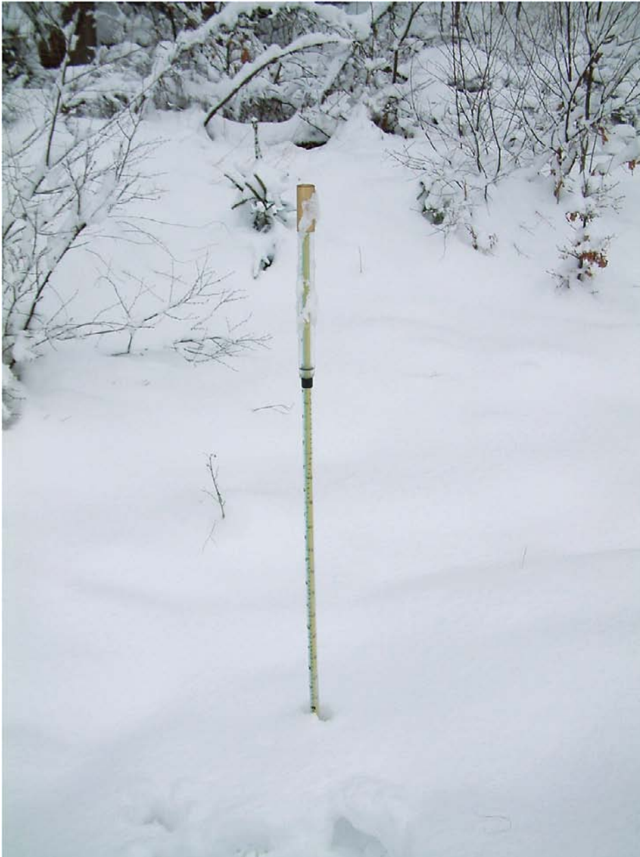
Figure 3-1. Measuring device for registration of depth of frost in the ground.
