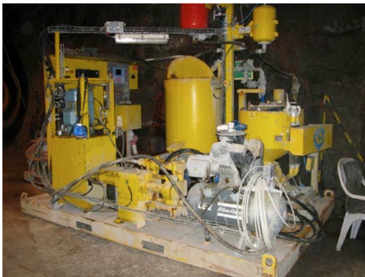
Figure 5-2. A grouting equipment, with mixer, agitator and pump for cement base grout or silica sol grout and also the control pane. Foto from SKB:s sealing project at great depth.
