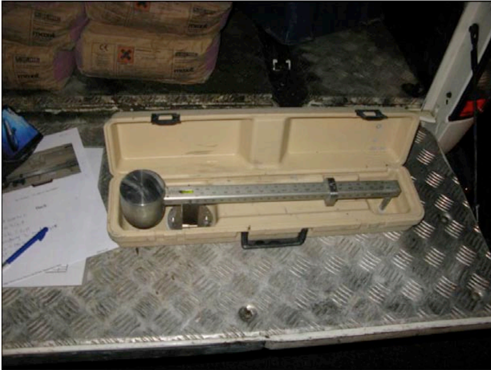
Figure 5-7. A “Mud balance” to check the specific weight.
