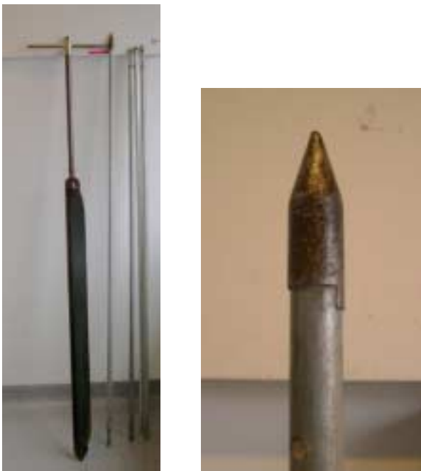
Figure 3-1. The coring equipment consists of a Russian peat corer, rods and a probe.
