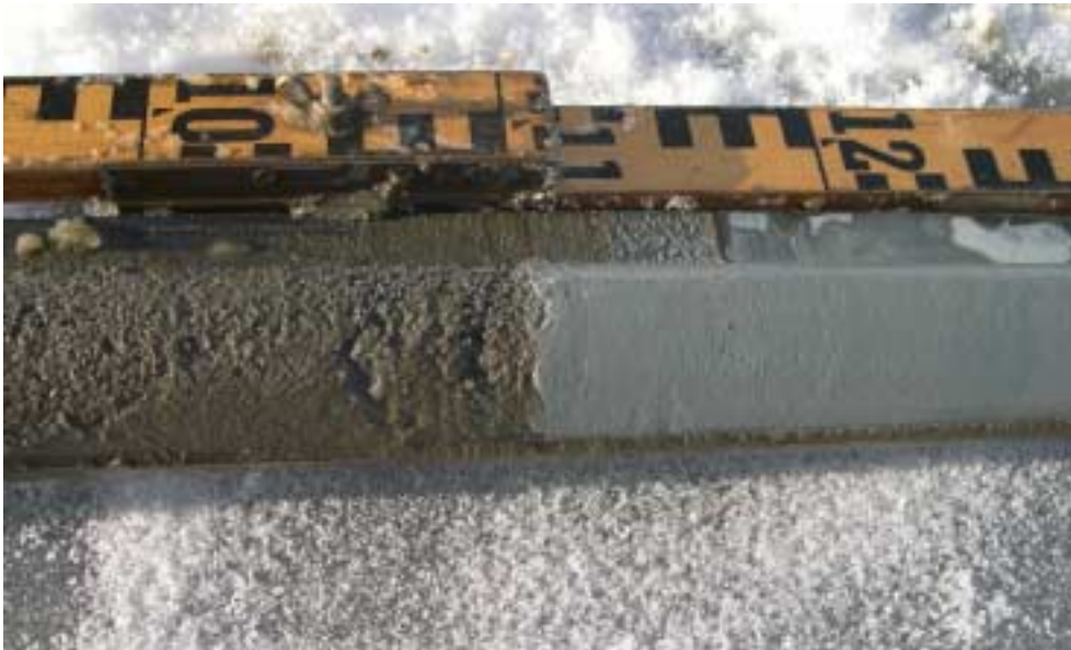
Figure 5-2. In Lake Eckarfjärden (lake No 26, coring site PFM004301), the typical erosive contact between the glacial clay and postglacial sand is recorded at 3.0 meter. Down is to the right in the picture.
