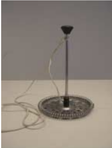
Figure 3-2. The Ising plummet. The water depth was measured with a home made plummet, constructed by J. Ising.
