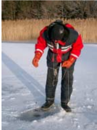
Figure 3-2. The Ising plummet. The water depth was measured with a home made plummet, constructed by J. Ising.
