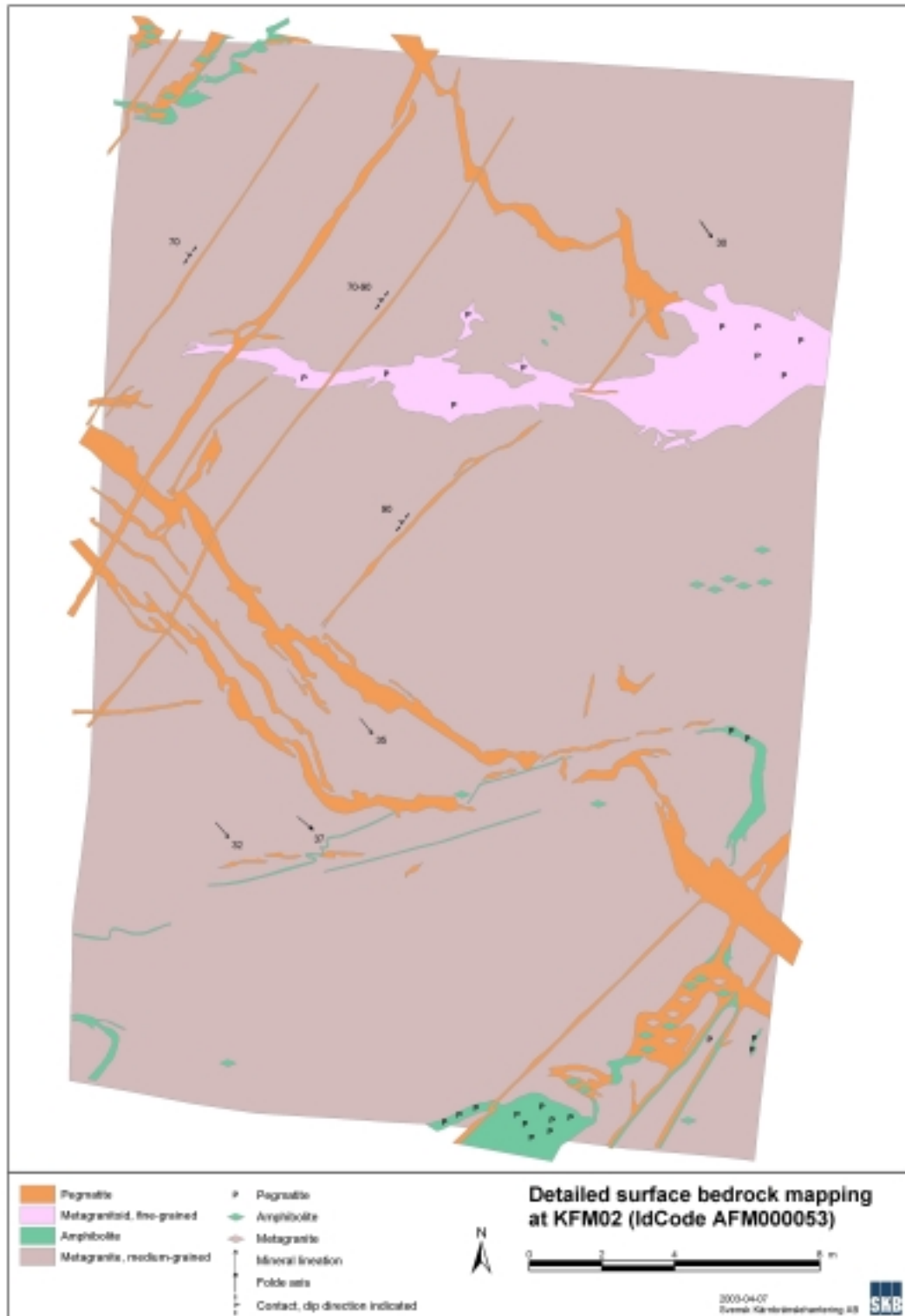
Figure A-1. Schematic geological map of stripped outcrop at drill site 2 (AFM000053).
