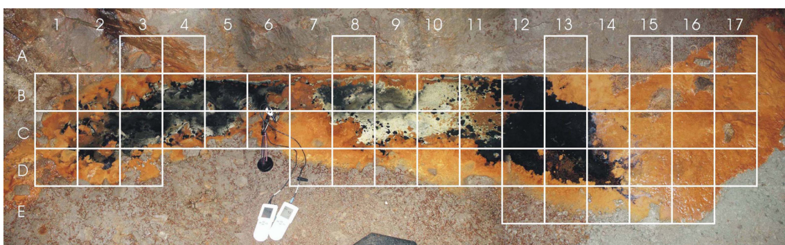
Figure 4-12. The 907 m ditch site is characterised by a shallow, elongated water pond that overflows into the main tunnel ditch to the right in the image. Brown material is BIOS. The black colour is from iron sulphide precipitates and the white material is calcium carbonate. The overlaid grid creates an organised environment and enables pH, oxygen and redox measurements in three dimensions (Field instruments shown in the bottom of the figure). Grid size is about 20 x 20 cm.
