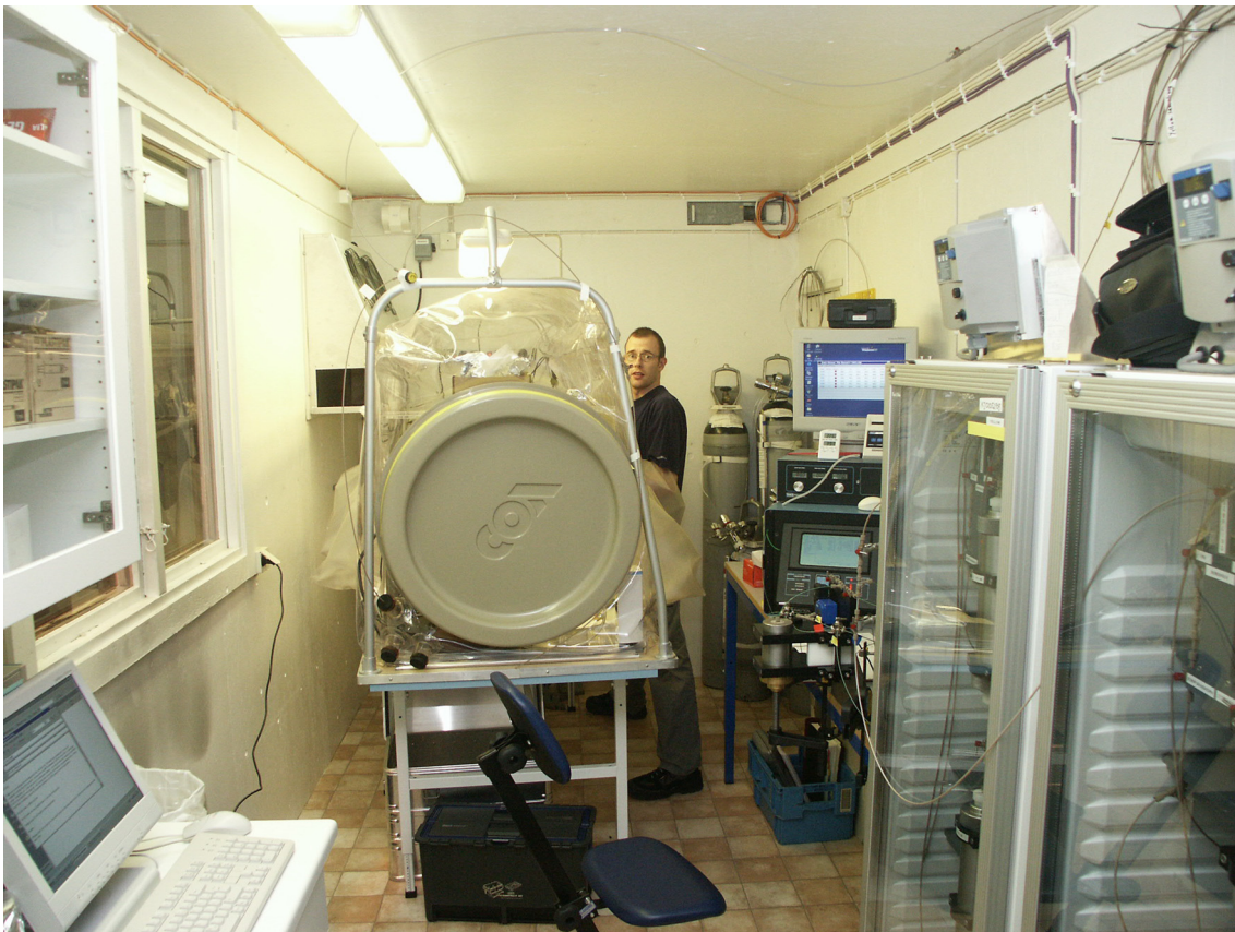
Figure 4-13. The Microbiology Laboratory environment at the MICROBE-450 m site is equipped with three circulation systems (right), an anaerobic box (forward), an in situ gas extractor, and a Kappa 5 gas chromatograph (right of the anaerobic box).
