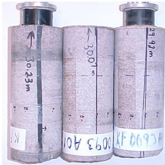
Figure A3-4. Photograph of three cores (29.92, 30.07 and 30.23) from the horizontal borehole (KF0093A01).
