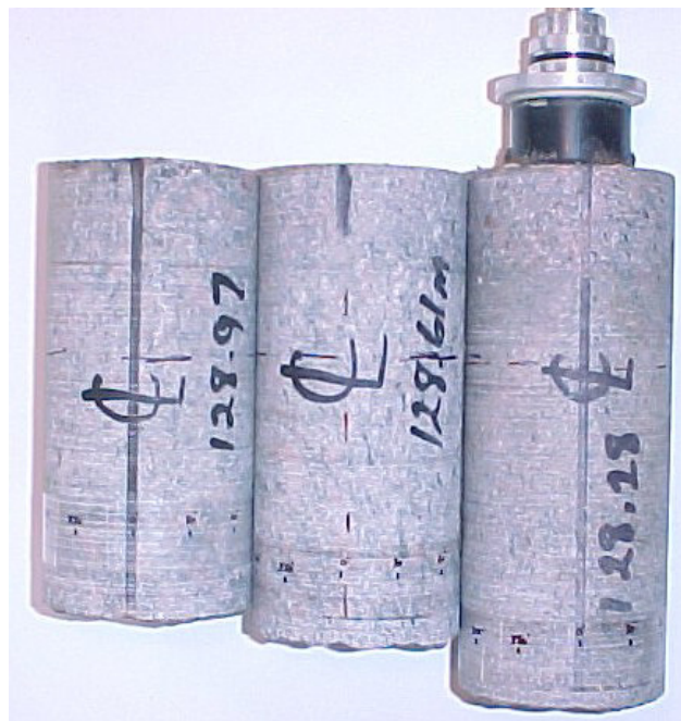
Figure A3-2. Photograph of three cores (128.28, 128.61 and 128.97) from the vertical borehole (KA2599G01).
