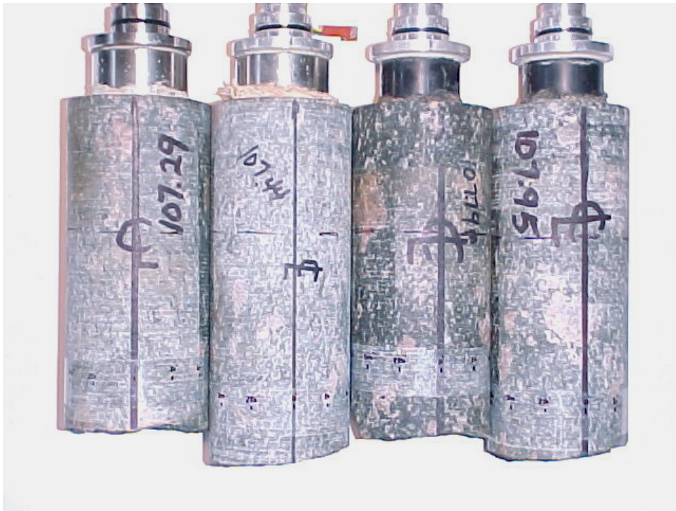
Figure A3-1. Photograph of four cores (107.29, 107.44, 107.79 and 107.95) from the vertical borehole (KA2599G01).
