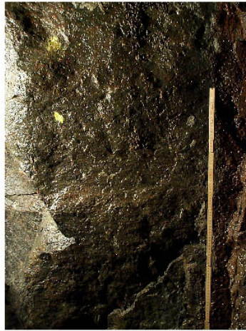
Photo 4: Structure1558m at 1566A (Site 1) Looking normal to the same fault plane. Steps and subhorizontal striations indicating dextral strike-slip. Width of photo ca.90cm.
