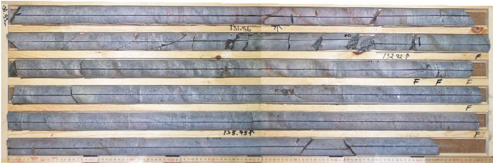
Photo 28: Section 1 No.34 and No.35 Open fractures along epidote-cataclasite with red alteration halo.
