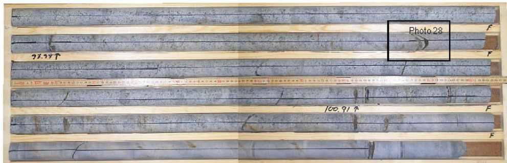
Photo 24: Section 1 whole view Length of box = 120cm.
