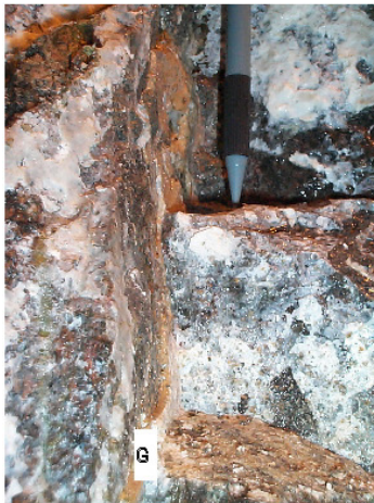
Photo 8: Structure 2198m at Niche 2198A (Site 3) Grout (G; light orange colour) injected into the master fault No. 1 with maximum thickness of 8mm. White material is re-precipitated grout. Width of photo ca. 15 cm.
