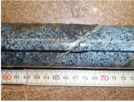
Photo 27: Section 1 No.32 A slightly open fracture along epidote vein with calcite coating.
