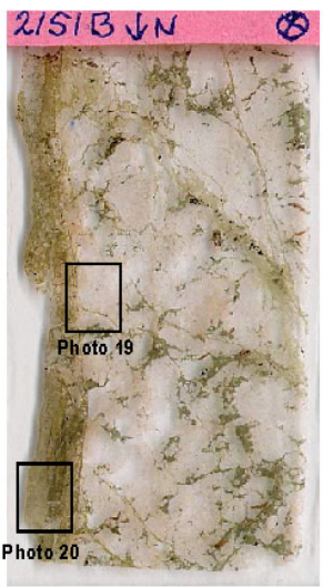
Photo 14: Prepared thin sections and location of microscopic photos See Figure 4-1 for explanation of orientation. Longer side of thin sections 45mm.
