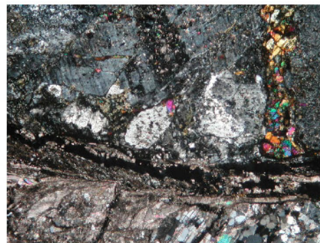
Photo 17: 1561B (width of photo ca. 5mm) Epidote vein (Epi) in the weakly crushed matrix is cut by the open fracture coated with fine drusy calcite (Cal).
