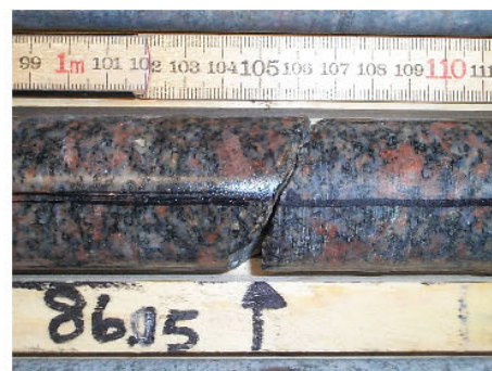
Photo 26: Section 1 No. 16 An open fracture with clay coating, no visible alteration and ductile deformation.
