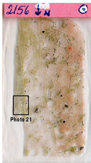
Photo 14: Prepared thin sections and location of microscopic photos See Figure 4-1 for explanation of orientation. Longer side of thin sections 45mm.
