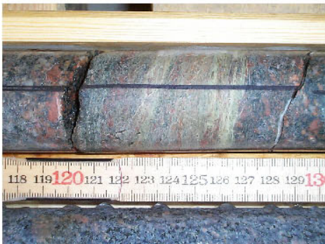
Photo 30: Section 2 No.7(left) and No.8 (right) Fractures at the rim of mylonite.
