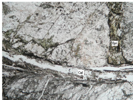
Photo 17: 1561B (width of photo ca. 5mm) Epidote vein (Epi) in the weakly crushed matrix is cut by the open fracture coated with fine drusy calcite (Cal).
