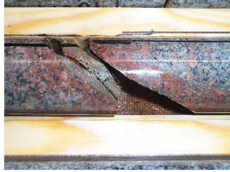
Photo 28: Section 1 No.34 and No.35 Open fractures along epidote-cataclasite with red alteration halo.
