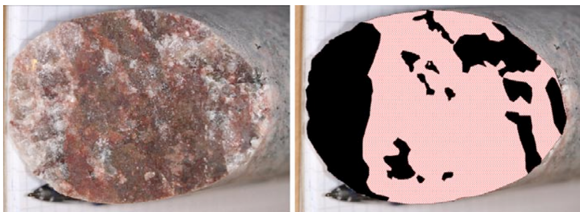
Figure 4-1. Image analysis of fracture surface coverage (KFM01D Adjusted sec up 736.322 m). The visible hematite coverage on the fracture surface (left picture) was estimated at 70%. Image analysis (right picture) yielded an absolute visible hematite coverage (cross hatched) of 63%.
