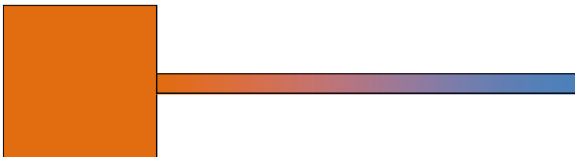
Figure A1-3. The walls of the container are impervious to water and to colloids. The clay in the container is fully water saturated and the fracture is filled with water.
