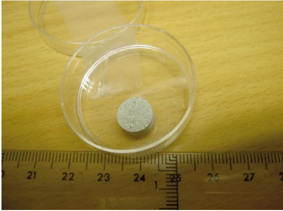
Figure 3-15. Disc shaped pellet used in expansion experiment.
