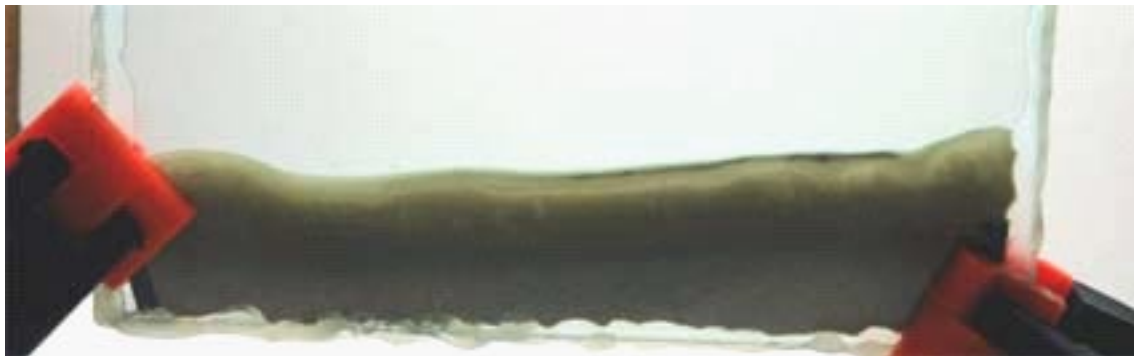
Figure 3-41. The swollen clay after two days. Width of slit is 13 cm.
