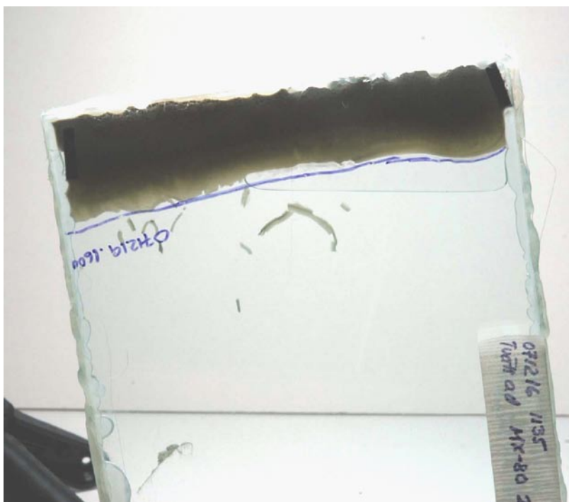
Figure 3-42. Falling worm like blobs hours after turning the slit upside down.
