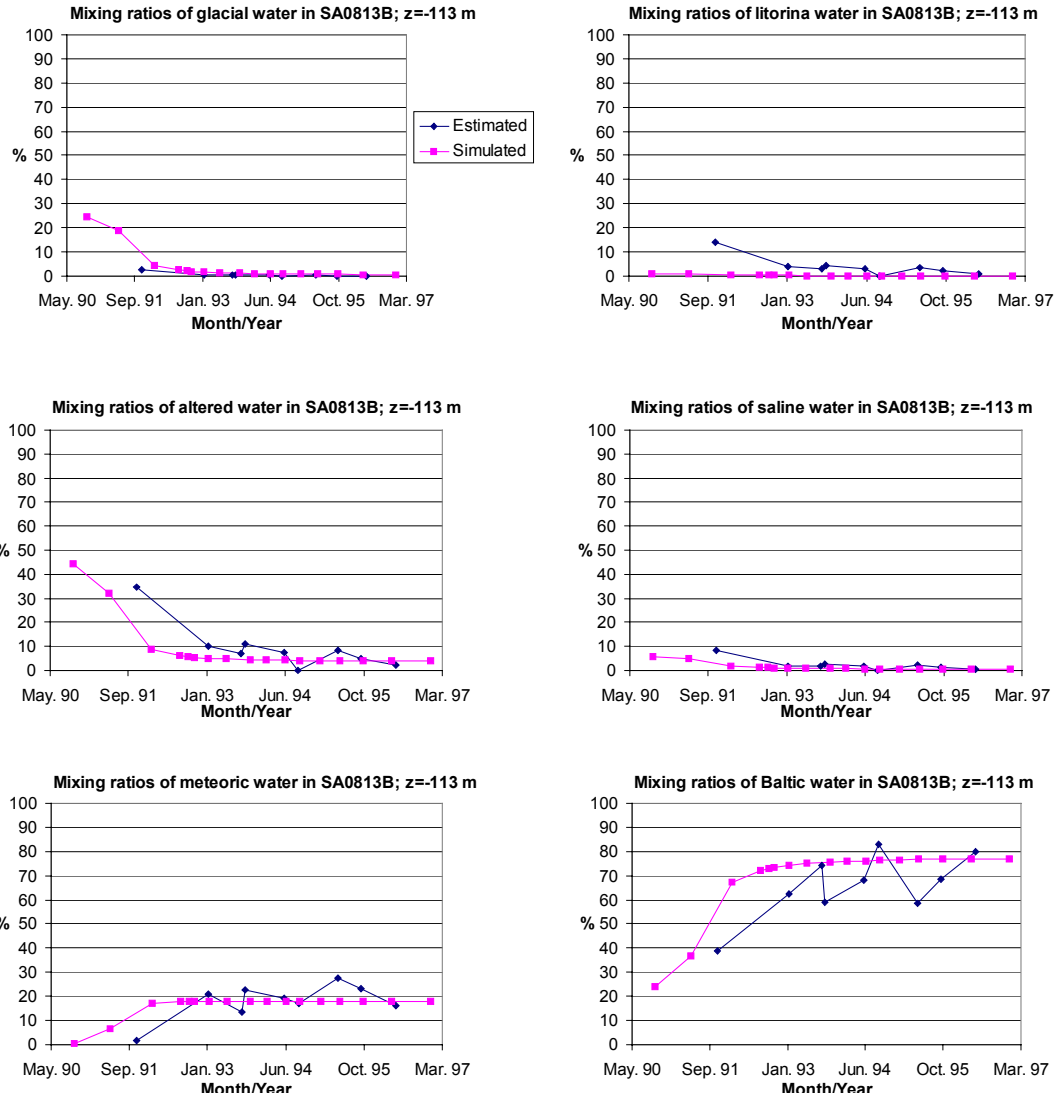
Figure 5.5. The mixing ratios of glacial, Litorina, altered, saline, meteoric and Baltic water in SA0813B as function of time.
