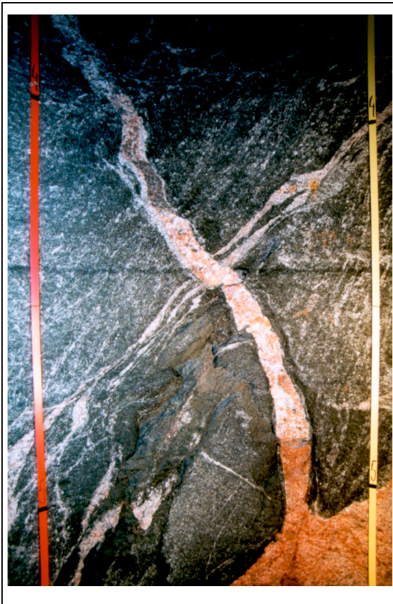
Appendix 14B. Photos from deposition hole DD0092G01. Part of the wall, section 4-5m, with an intersection between pegmatite (pinkish white) and fine-grained granite/pegmatite hybrid rock. Surrounding rock types are greenstones (grey-dark grey). Photo: Lars Andersson, SKB.
