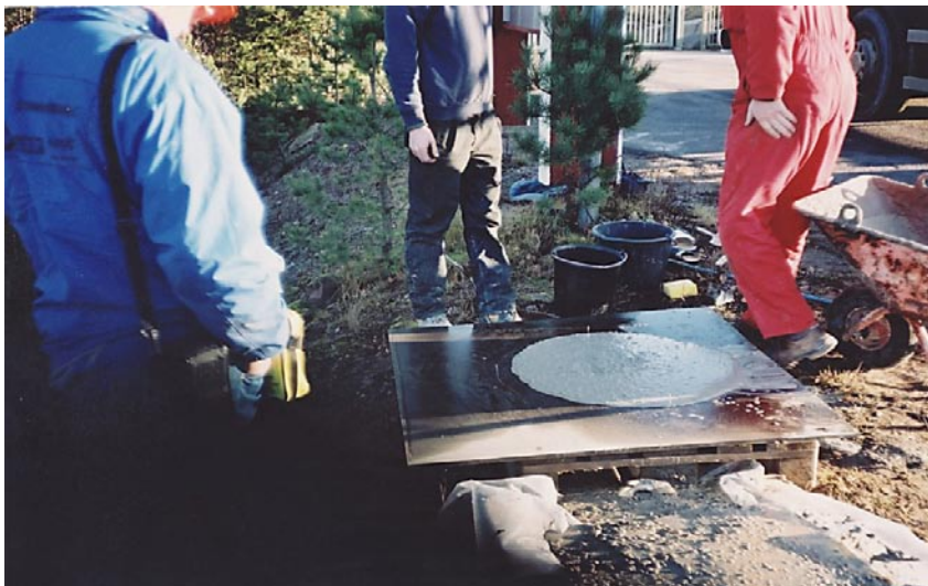
Figure 5-13. Slump tests at arrival to Äspö.
