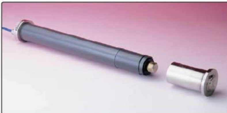
Figure 7-1. Geokon Model 4400 joint meter.
