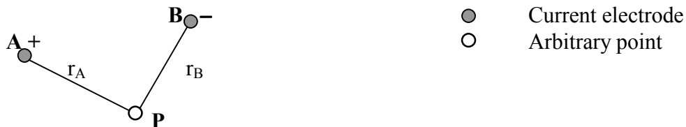
Figure 4-3 Two oppositely charged electrodes and an arbitrary point in an homogenous medium.
