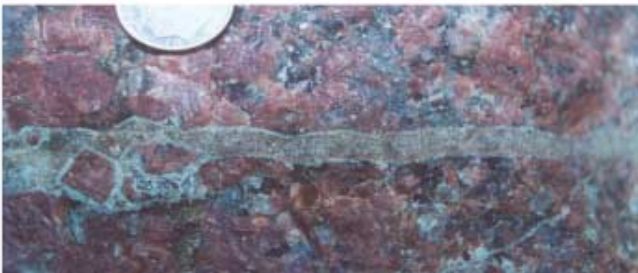
Figure 5-25. Sandstone dykes from the Kråkemåla quarry showing a sandstone matrix supporting clasts of granite. The dyke edges and the margins of the granite clasts are clearly mineralised. The dykes pre-date the mineralisation which is thought to be of Permian age.
