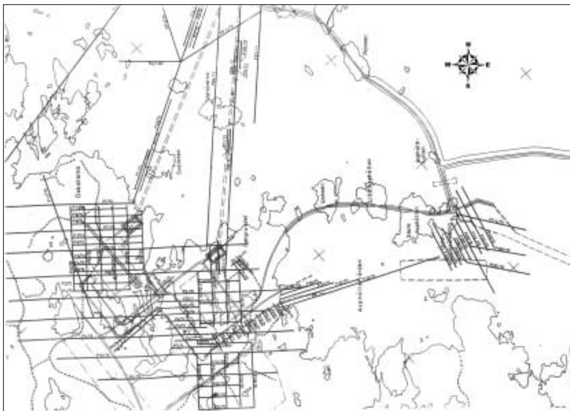
Figure 2-4. Above: Example of an inventory database entry from the Vattenfall Archive, describing an overview drawing of seismic profiling performed in the Forsmark construction area. Below: Map (an extract from the actual drawing), showing the Forsmark construction area and the location of seismic profiles performed up to 1976.
